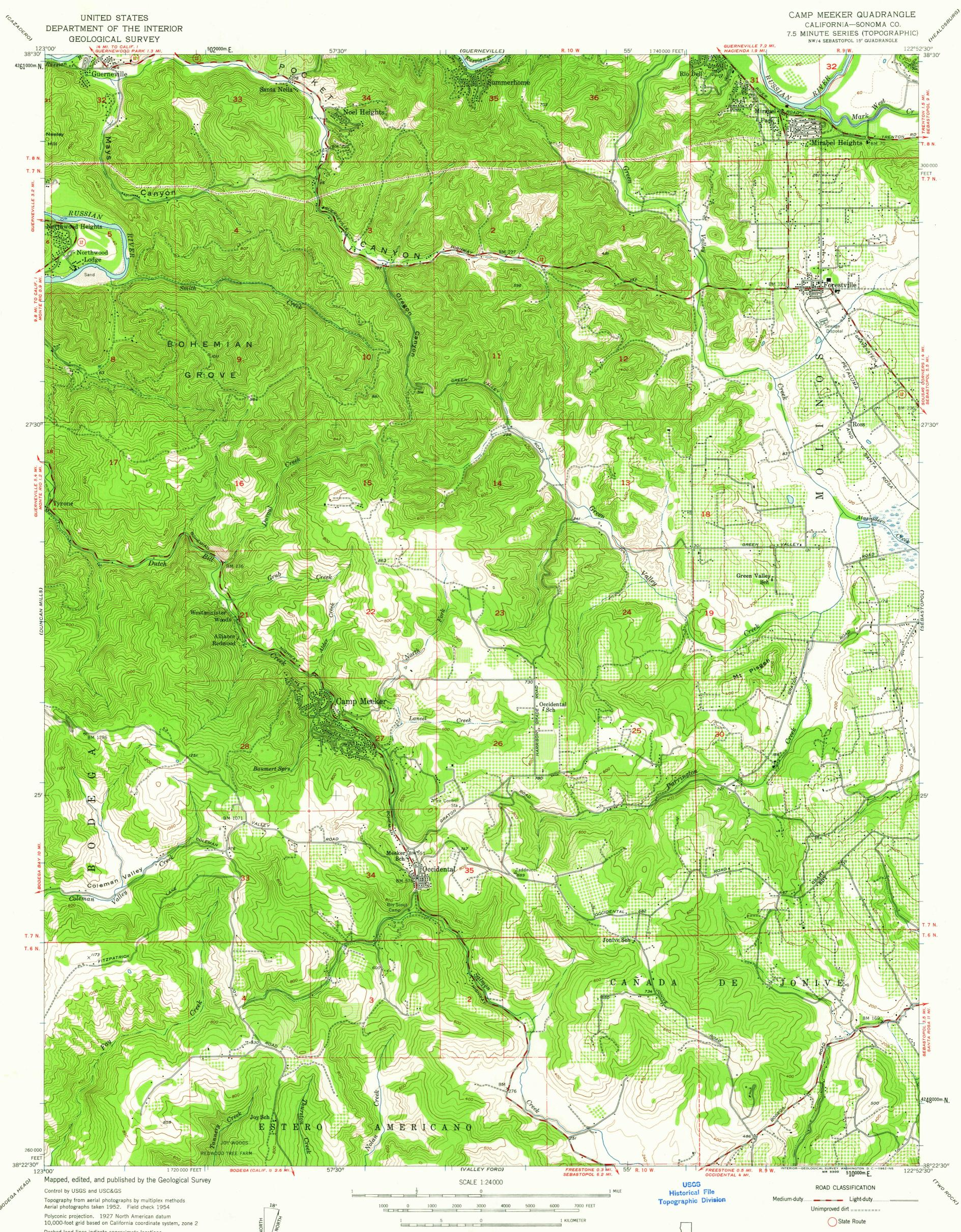
10,000-foot grid based on California coordinate system, zone 2 Dashed land lines indicate approximate locations Unchecked elevations are shown in brown 1000-meter Universal Transverse Mercator grid ticks, zone 10, shown in blue
