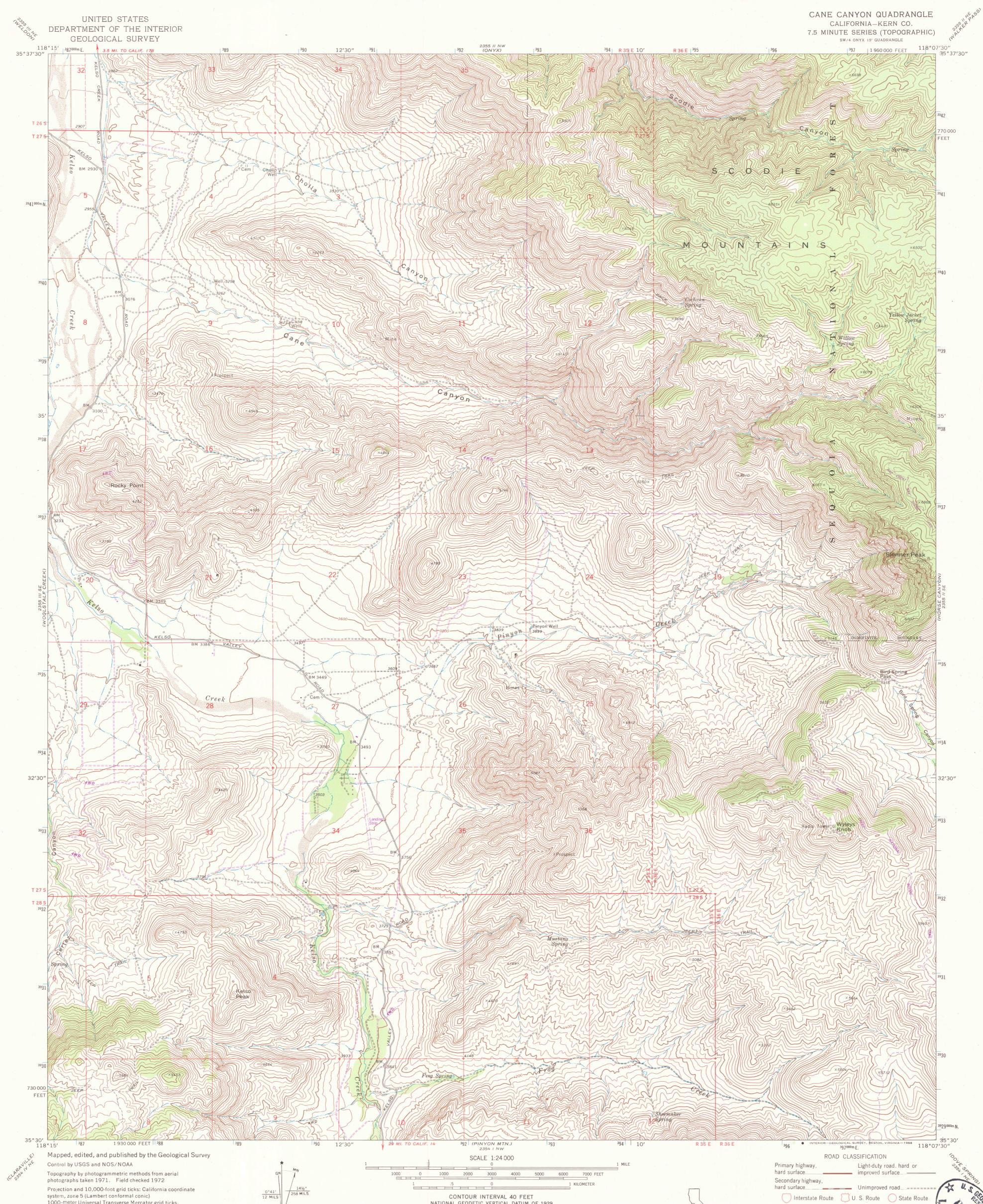
Projection and 10,000-foot grid ticks: California coordinate system, zone 5 (Lambert conformal conic) 1000-meter Universal Transverse Mercator grid ticks, zone 11, shown in blue. 1927 North American datum To place on the predicted North American Datum 1983 move the projection lines 7 meters north and 83 meters east as shown by dashed corner ticks
