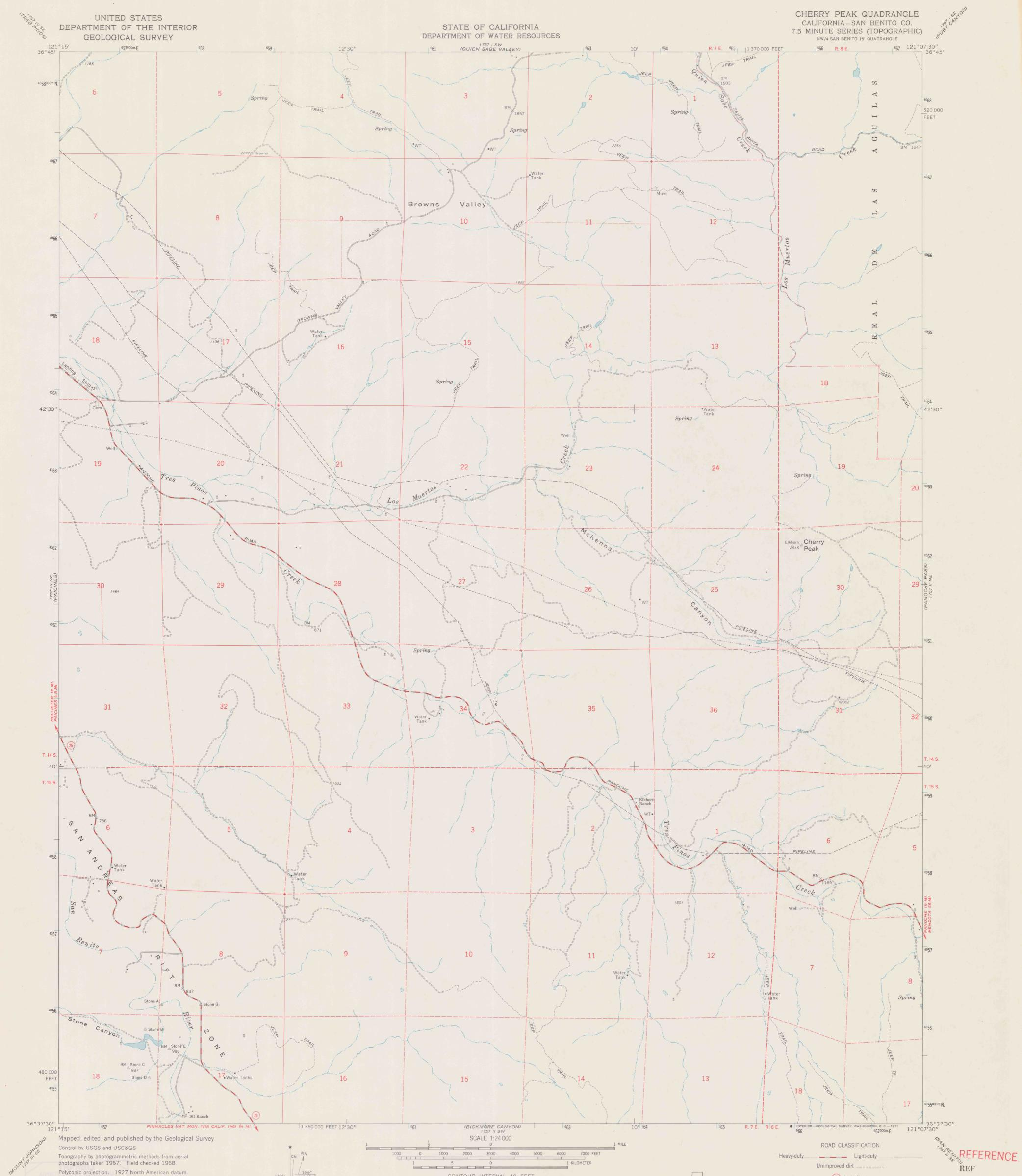
Topography by photogrammetric methods from aerial photographs taken 1967. Field checked 1968 Polyconic projection. 1927 North American datum 10,000-foot grid based on California coordinate system, zone 4 1000-meter Universal Transverse Mercator grid ticks, zone 10, shown in blue
