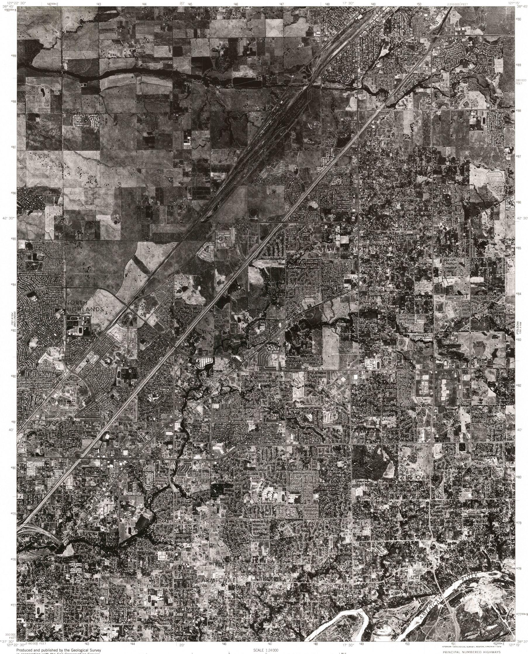
Produced and published by the Geological Survey in cooperation with the Soil Conservation Service Orthophotograph prepared from 1:80 000-scale aerial photographs taken August 29, 1975 Projection and 10,000-foot grid ticks: California coordinate system, zone 2 (Lambert conformal conic) 1000-meter Universal Transverse Mercator grid ticks, zone 10. 1927 North American datum
