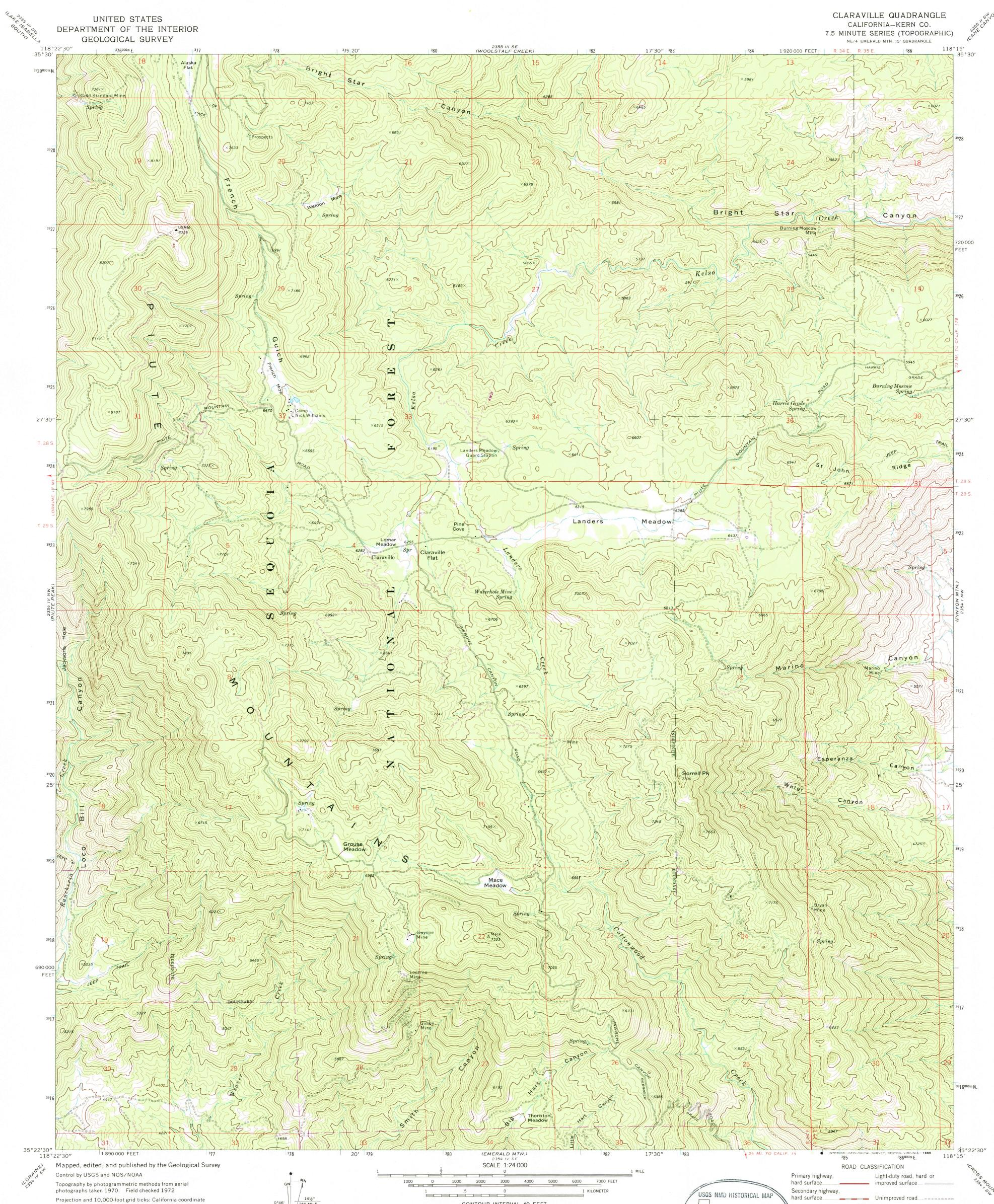
system, zone 5, (Lambert conformal conic) 1000-meter Universal Transverse Mercator grid ticks, zone 11, shown in blue. 1927 North American datum To place on the predicted North American Datum 1983 move the projection lines 7 meters north and 84 meters east as shown by dashed corner ticks
