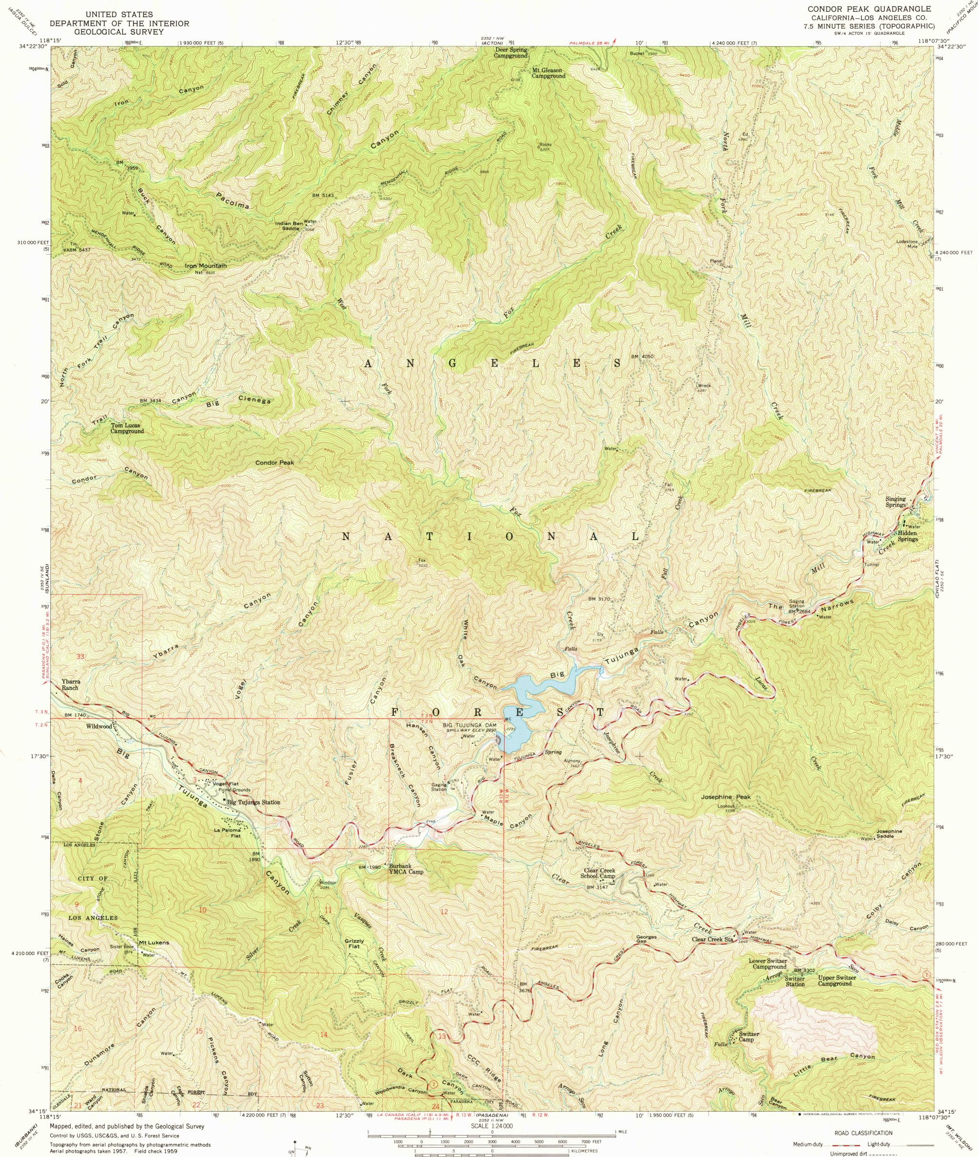
Polyconic projection. 1927 North American datum 10,000-foot grids based on California coordinate system, zones 7 and 5 1000-metre Universal Transverse Mercator grid ticks, zone 11, shown in blue
