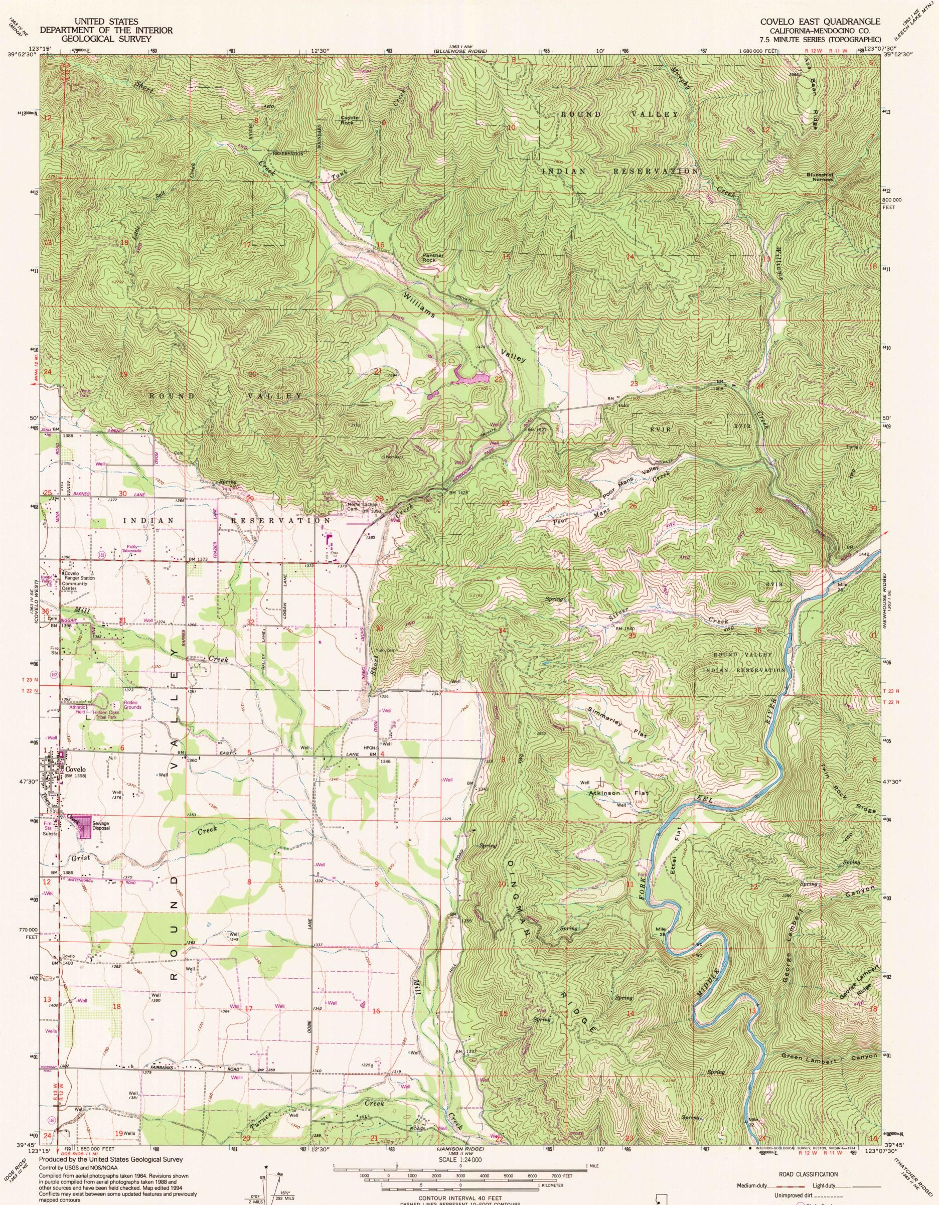
North American Datum of 1927 (NAD 27). Projection and 10 000-foot ticks : California Coordinate System, zone 2 (Lambert Conformal Conic) Blue 1000-meter Universal Transverse Mercator ticks, zone 10 North American Datum of 1983 (NAD 83) is shown by dashed corner ticks. The values of the shift between NAD 27 and NAD 83 for 7.5-minute intersections are obtainable from National Geodetic Survey NADCON software
