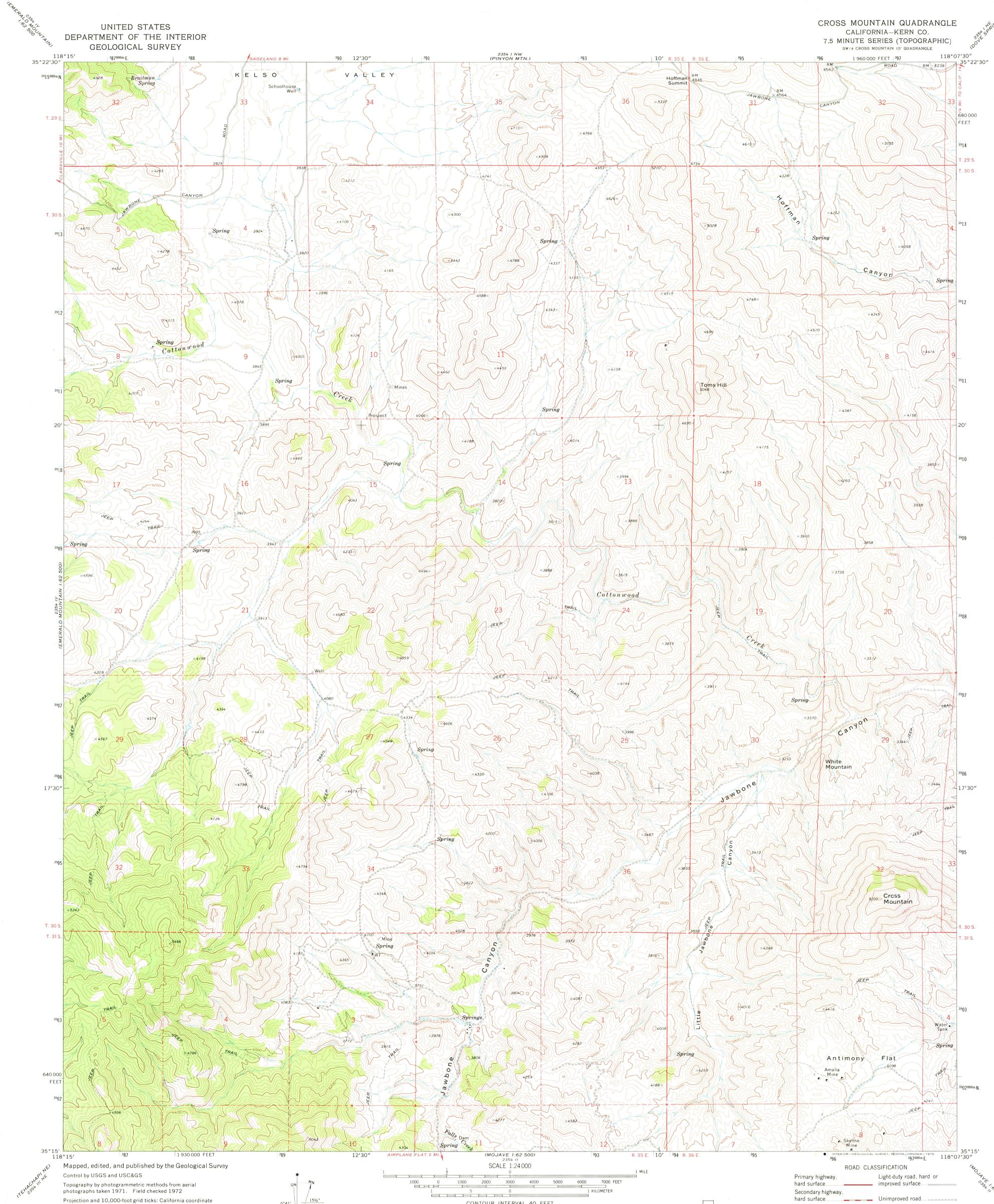
system, zone 5 (Lambert conformal conic) 1000-meter Universal Transverse Mercator grid ticks, zone 11, shown in blue. 1927 North American datum Fine red dashed lines indicate selected fence lines
