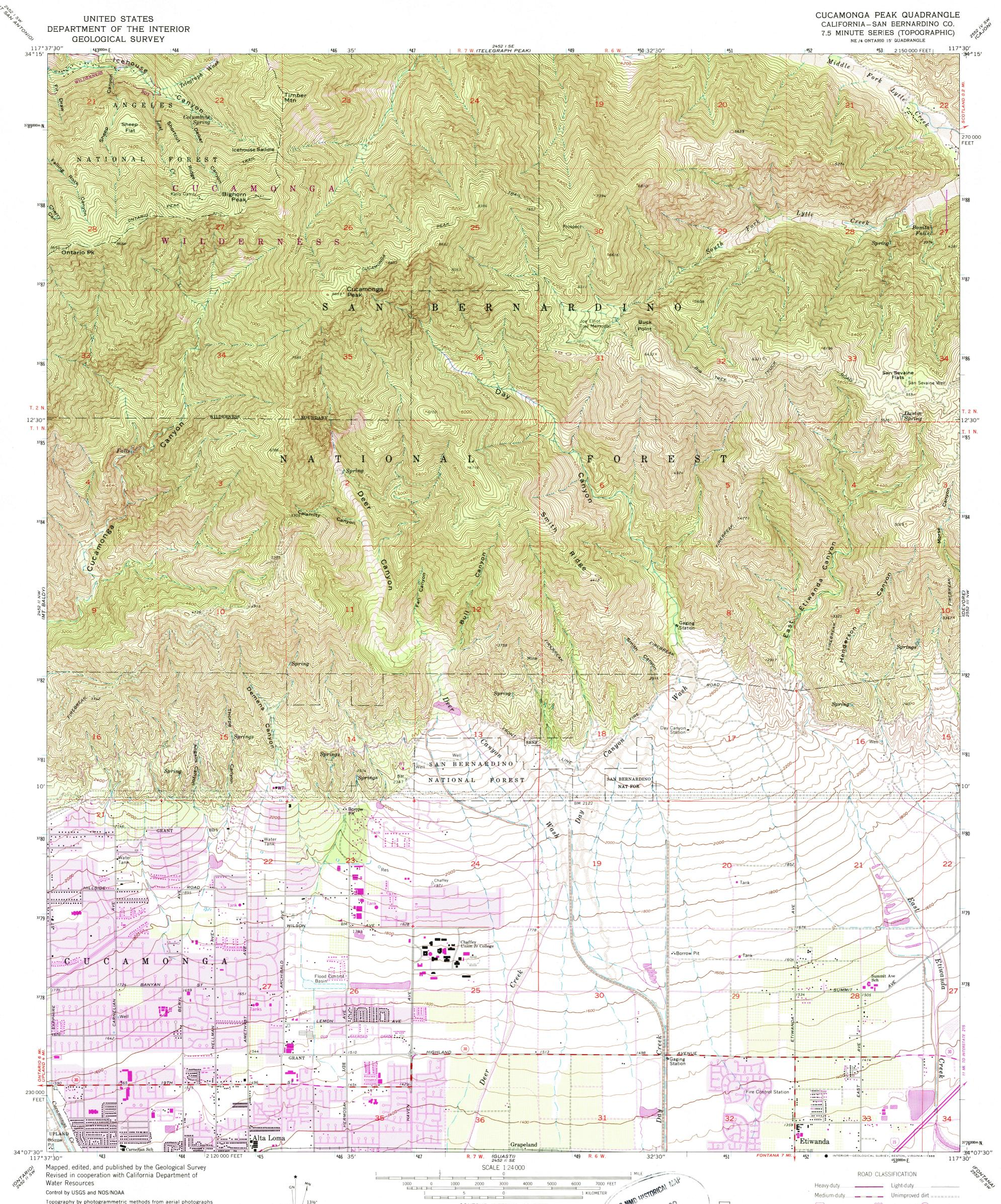
lopography by photogrammetric methods from aerial photographs taken 1952 and planetable surveys 1933. Field checked 1953 Revised from aerial photographs taken 1966. Field checked 1966
