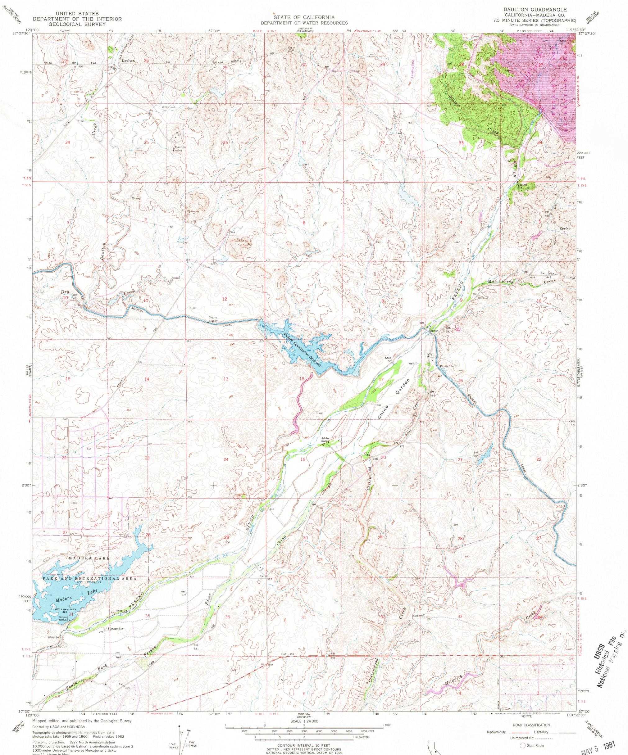
10,000-foot grids based on California coordinate system, zone 3 1000-meter Universal Transverse Mercator grid ticks, zone 11, shown in blue To place on the predicted North American Datum 1983, move the projection lines 9 meters north and 88 meters east as shown by dashed corner ticks
