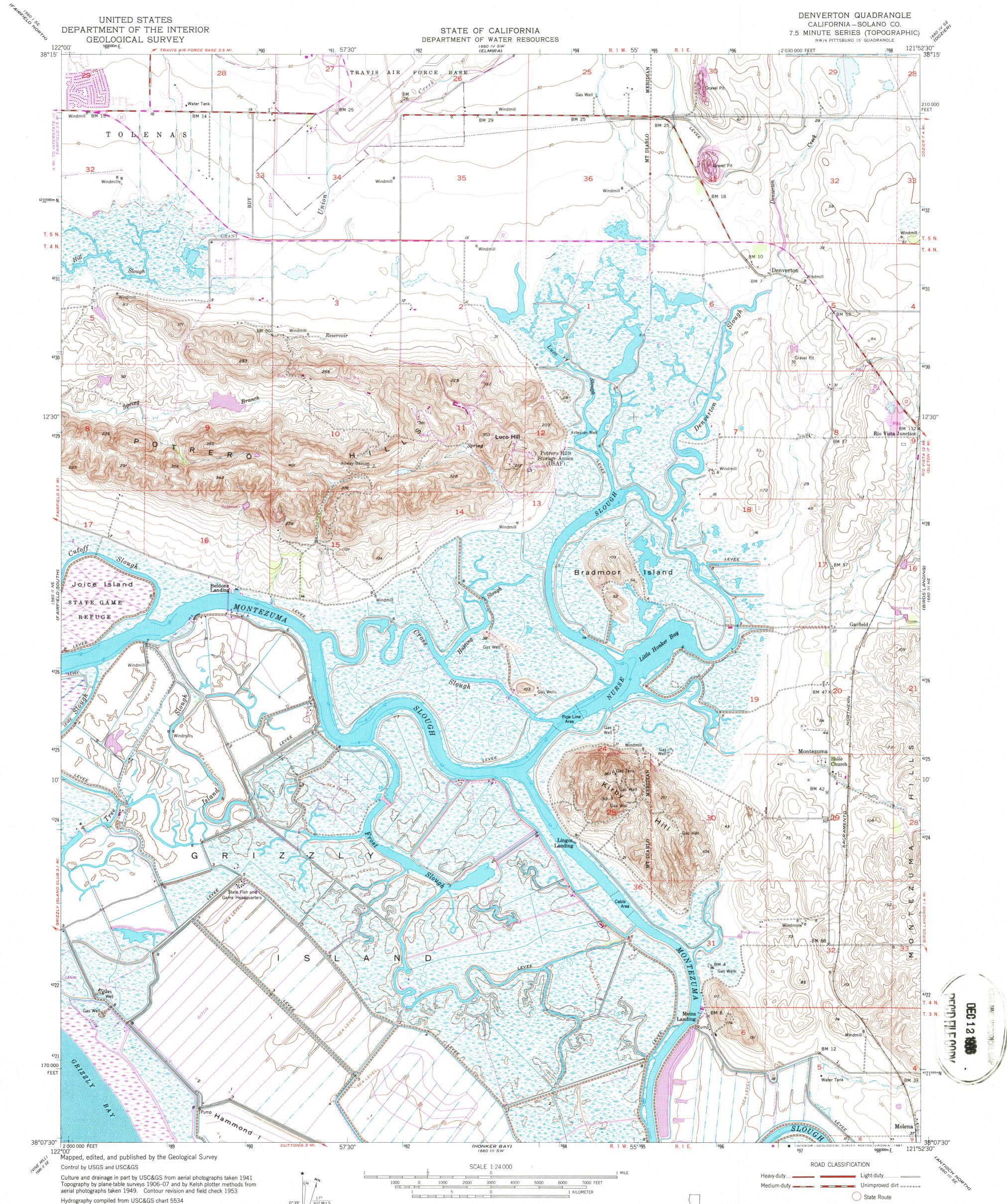
Polyconic projection 10,000-foot grid based on California coordinate system, zone 2 1000-meter Universal Transverse Mercator grid ticks, zone 10 shown in blue. 1927 North American Datum To place on the predicted North American Datum 1983 move the projection lines 14 meters north and 94 meters east as shown by dashed corner ticks
