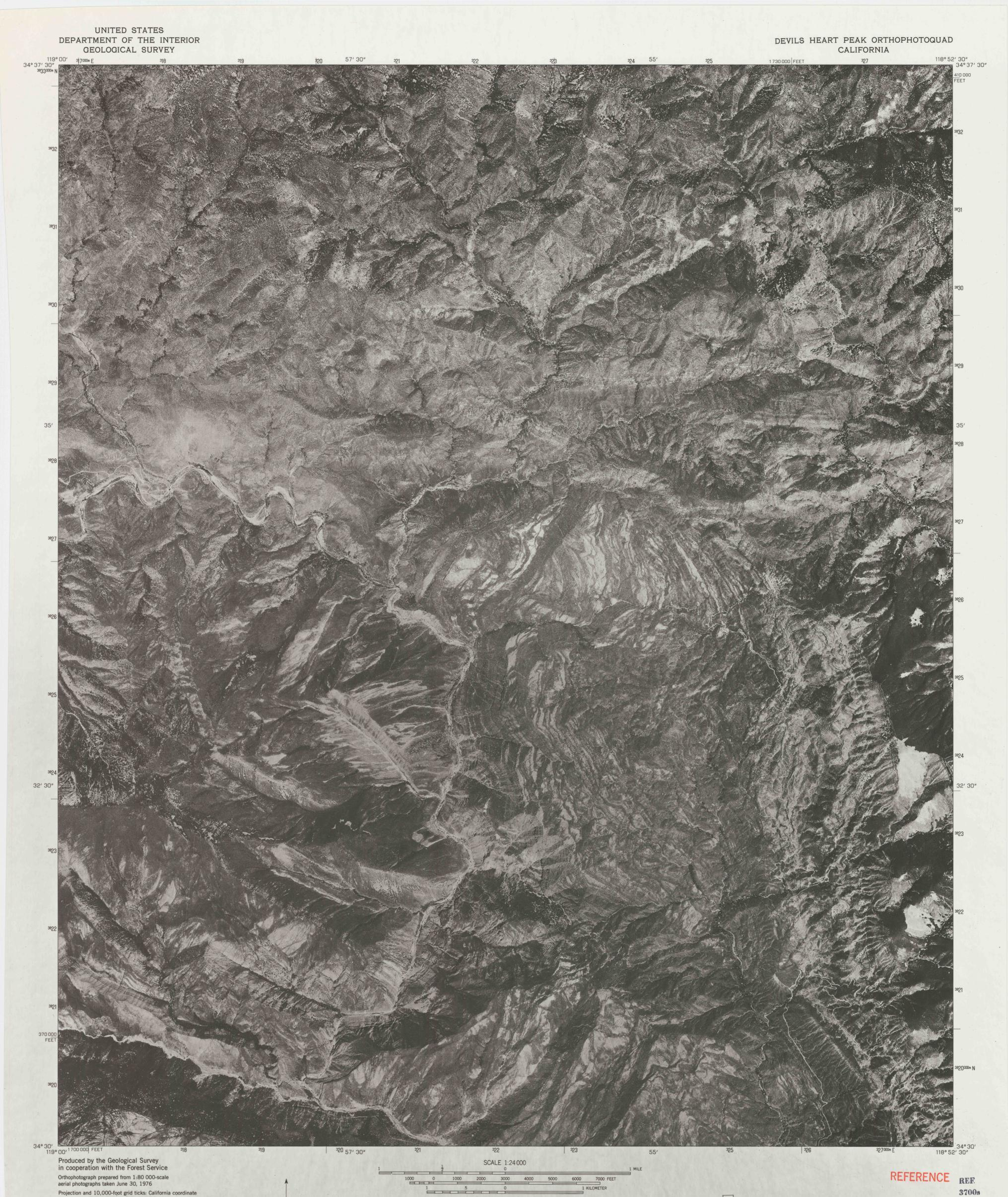
Projection and 10,000-foot grid ticks: California coordinate system, zone 5 (Lambert conformal conic) 1000-meter Universal Transverse Mercator grid ticks, zone 11. 1927 North American datum
