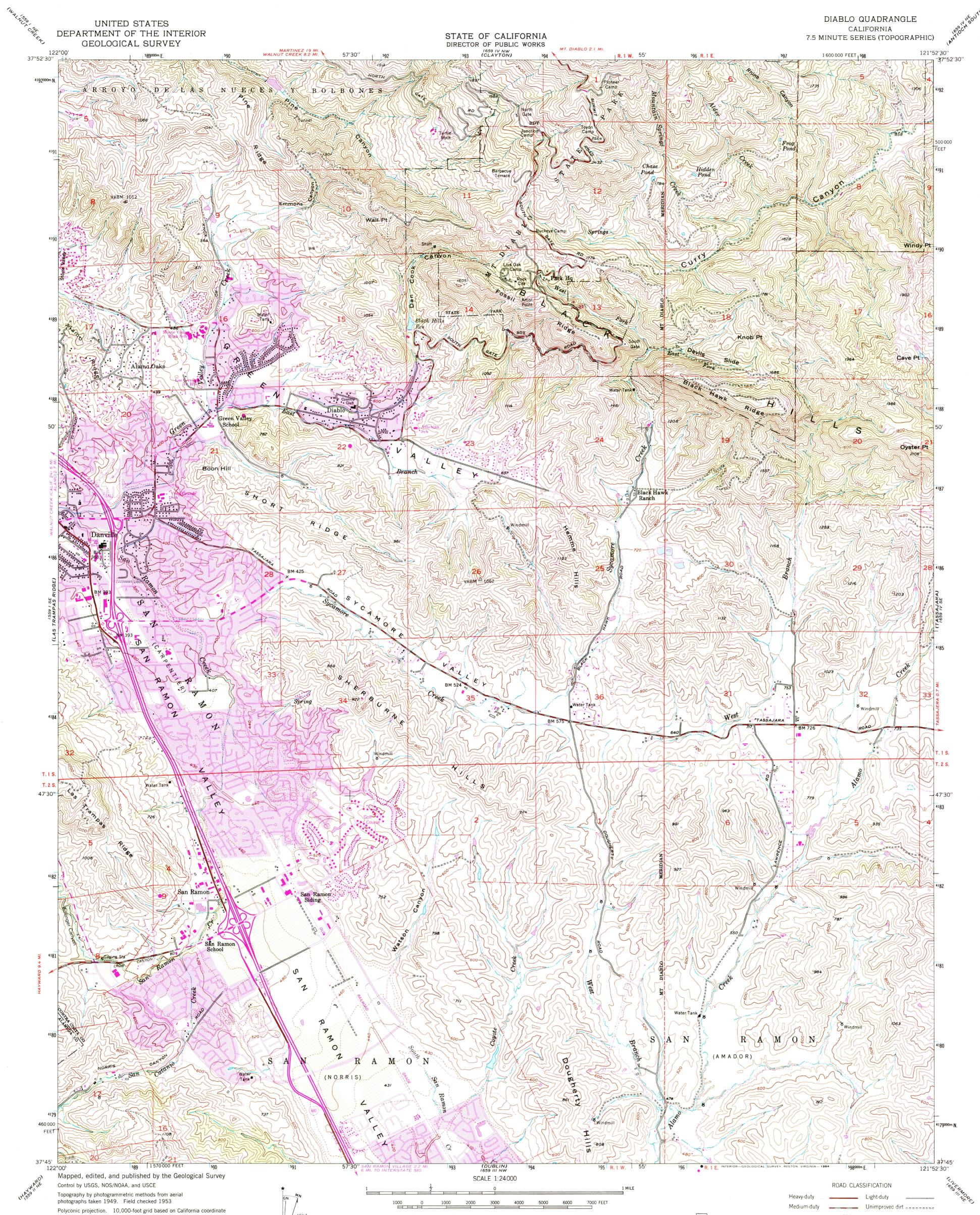
Polyconic projection. 10,000-foot grid based on California coordinate system, zone 3. 1000-meter Universal Transverse Mercator grid ticks, zone 10, shown in blue. 1927 North American Datum. To place on the predicted North American Datum 1983 move the projection lines 14 meters north and 94 meters east as shown by dashed corner ticks
