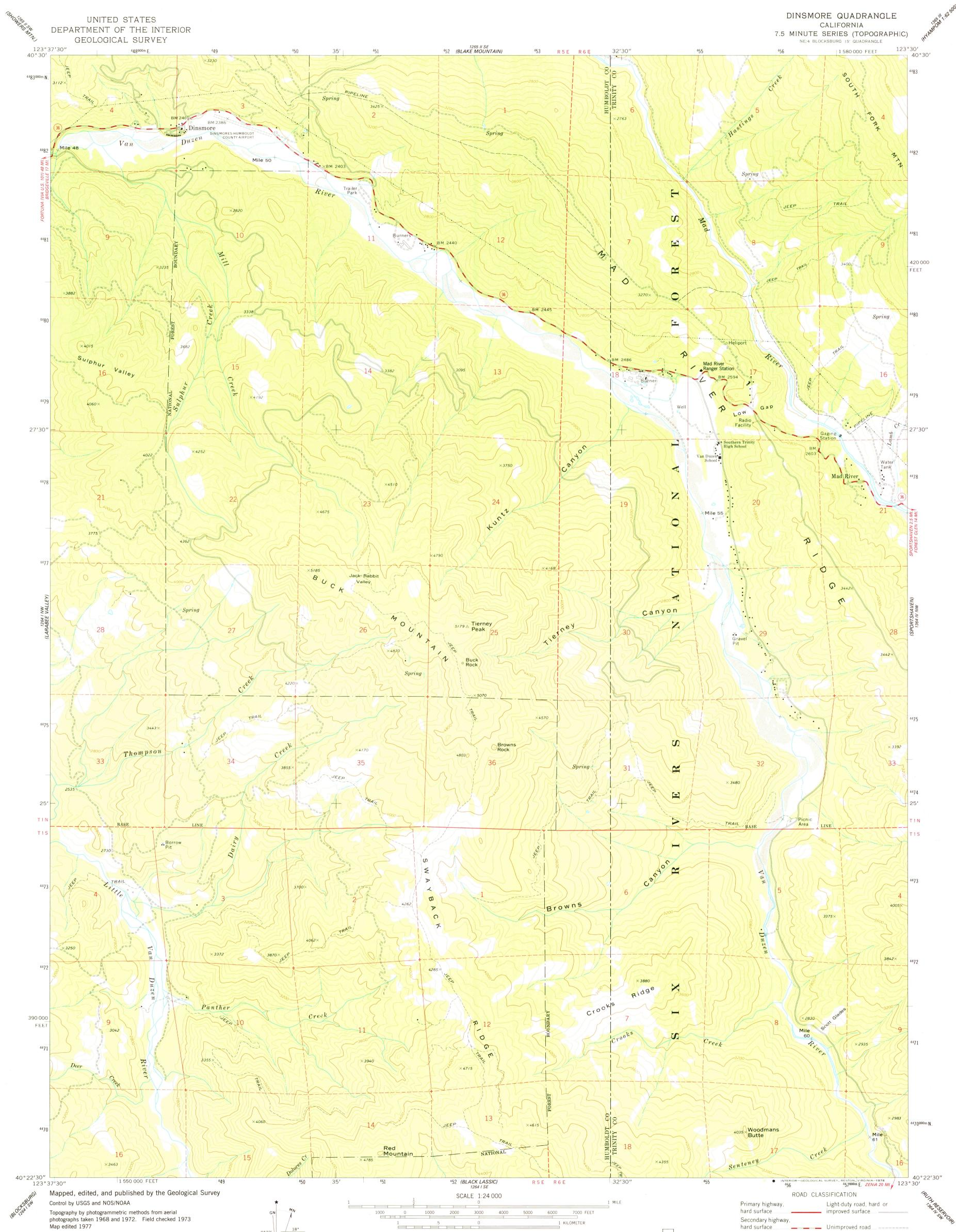
Projection and 10,000-foot grid ticks: California coordinate system, zone 1 (Lambert conformal conic) 1000-meter Universal Transverse Mercator grid ticks, zone 10, shown in blue. 1927 North American datum
