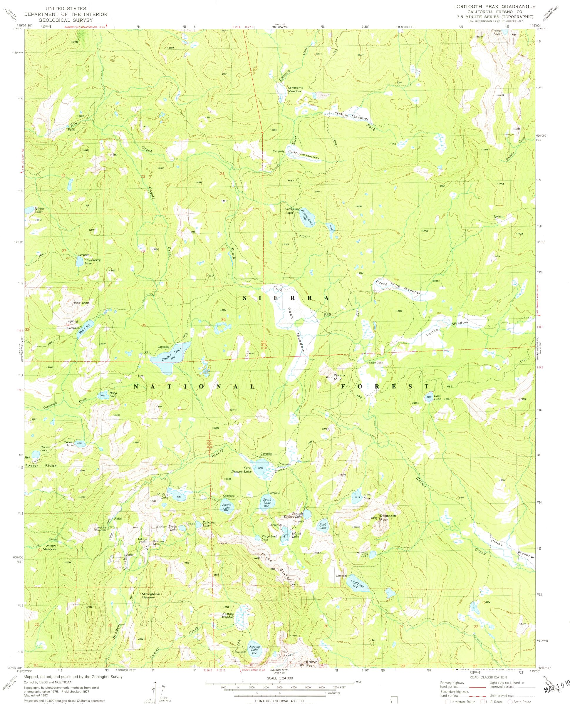
Projection and 10,000-foot grid ticks: California coordinate system, zone 4 (Lambert conformal conic) 1000-meter Universal Transverse Mercator grid, zone 11 1927 North American Datum To place on the predicted North American Datum 1983 move the projection lines 10 meters north and 85 meters east as shown by dashed corner ticks Where omitted, landlines have not been established or are not shown because of insufficient data There may be private inholdings within the boundaries of
