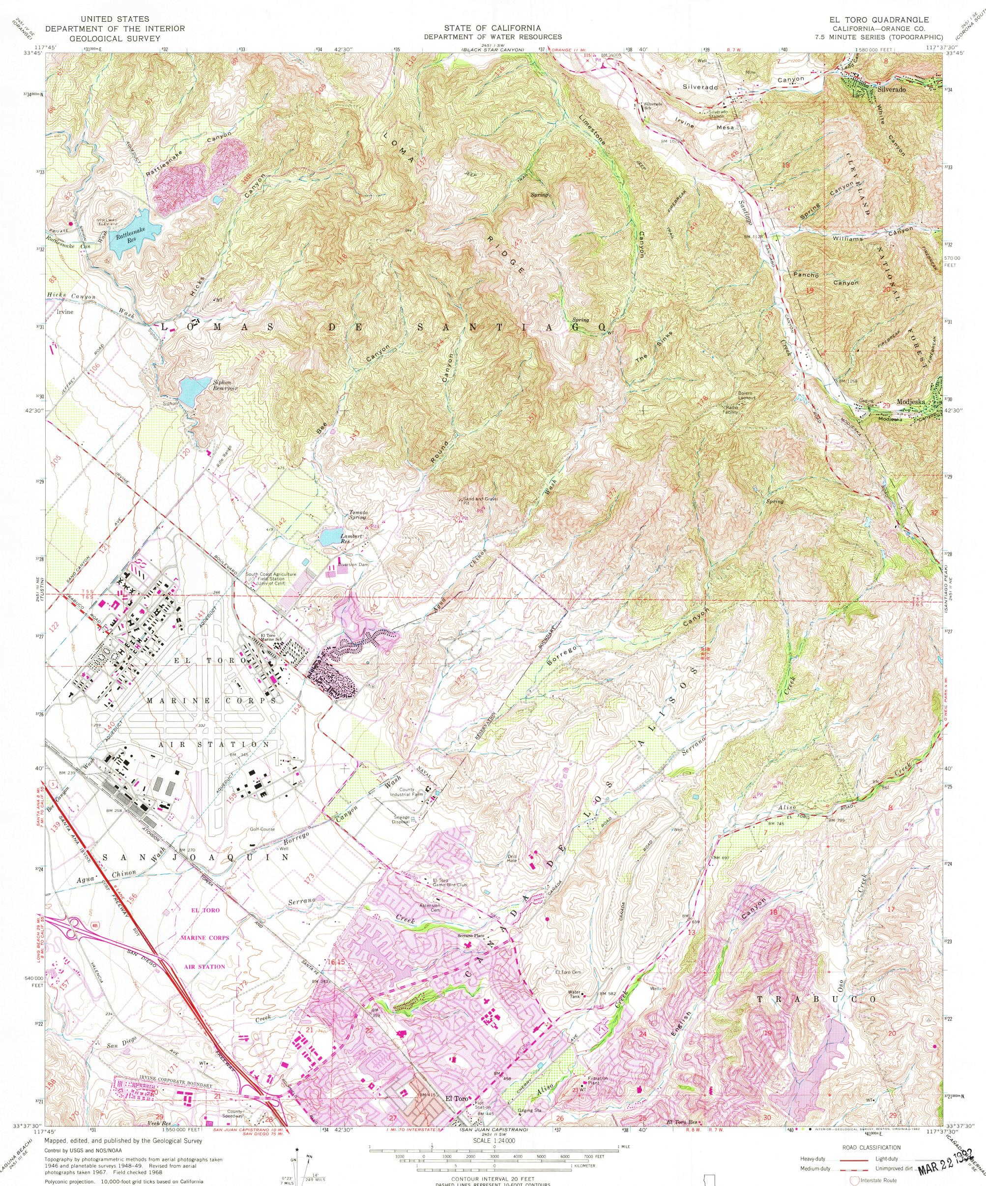
Polyconic projection. 10,000-foot grid ticks based on California coordinate system, zone 6. 1000-meter Universal Transverse Mercator grid ticks, zone 11, shown in blue. 1927 North American Datum. To place on the predicted North American Datum 1983 move the projection lines 83 meters east as shown by dashed corner ticks
