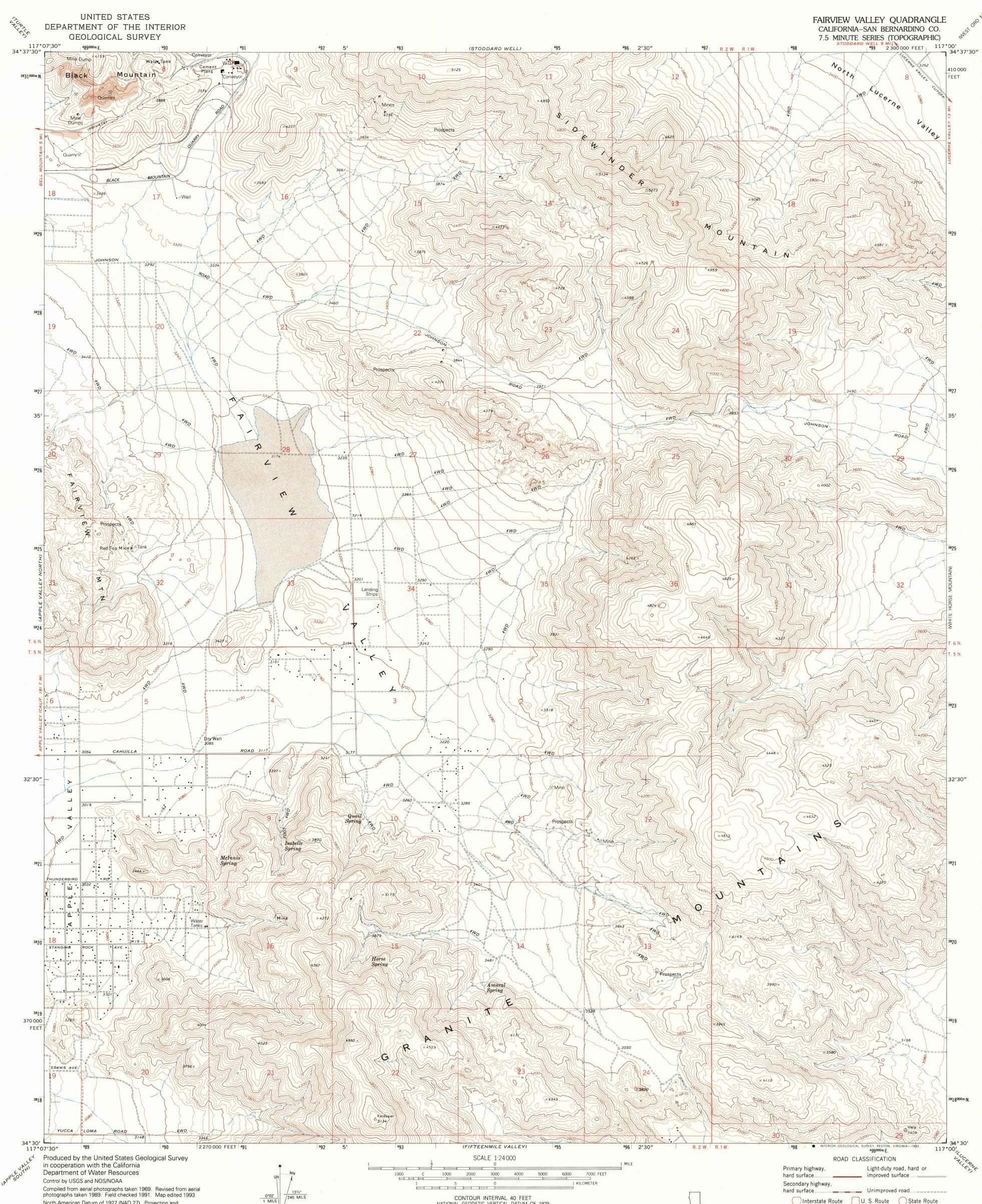
North American Datum of 1927 (NAD 27). Projection and 10000-foot grid ticks: California Coordinate System, zone 5 (Lambert Conformal Conic). Blue 1000-meter Universal Transverse Mercator grid ticks, zone 11 The difference between NAD 27 and North American Datum of 1983 (NAD 83) for 7.5 minute intersections is given in USGS Bulletin 1875. The NAD 83 is shown by dashed corner ticks
