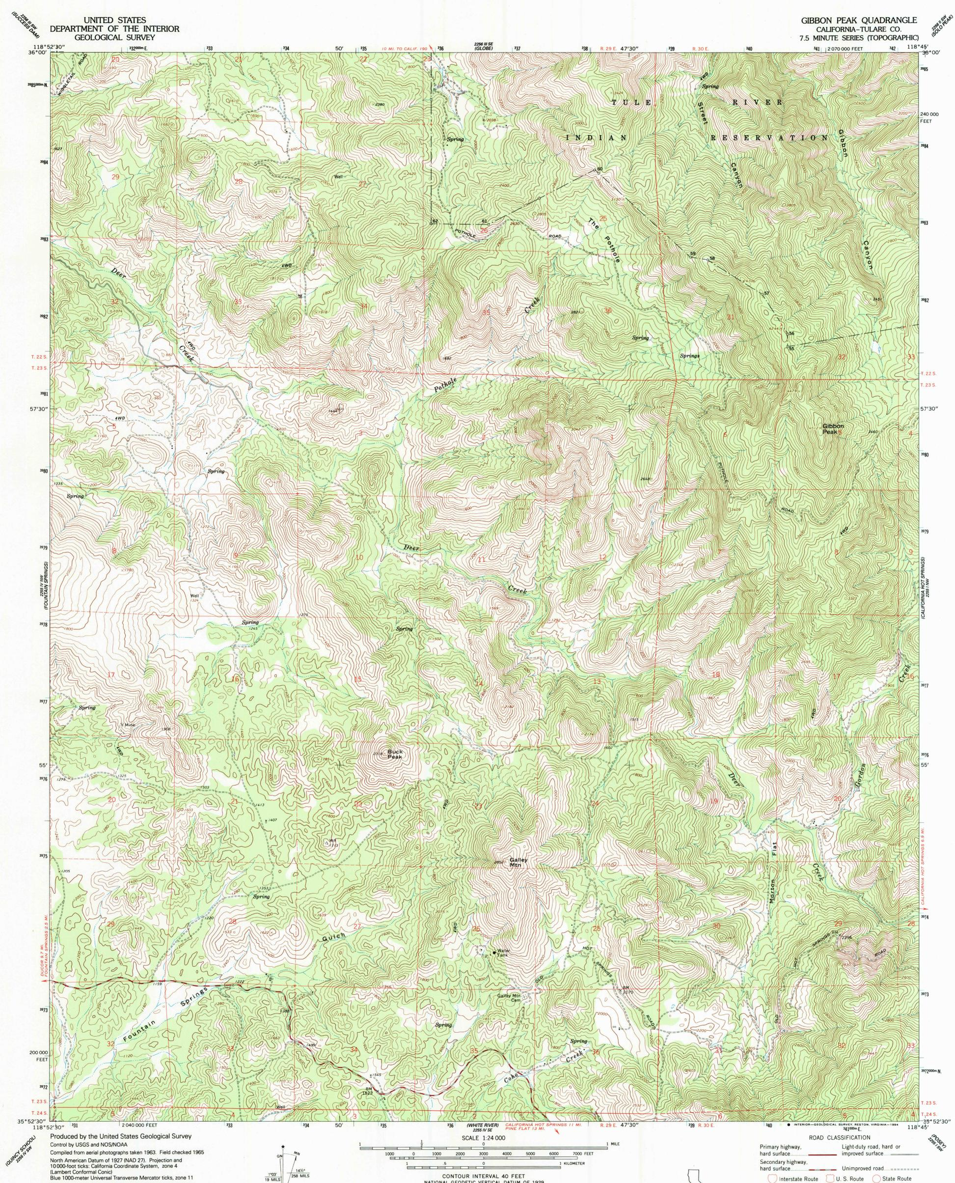
Blue 1000-meter Universal Transverse Mercator ticks, zone 11 North American Datum of 1983 (NAD 83) is shown by dashed corner ticks. The values of the shift between NAD 27 and NAD 83 for 7.5-minute intersections are obtainable from National Geodetic Survey NADCON software
