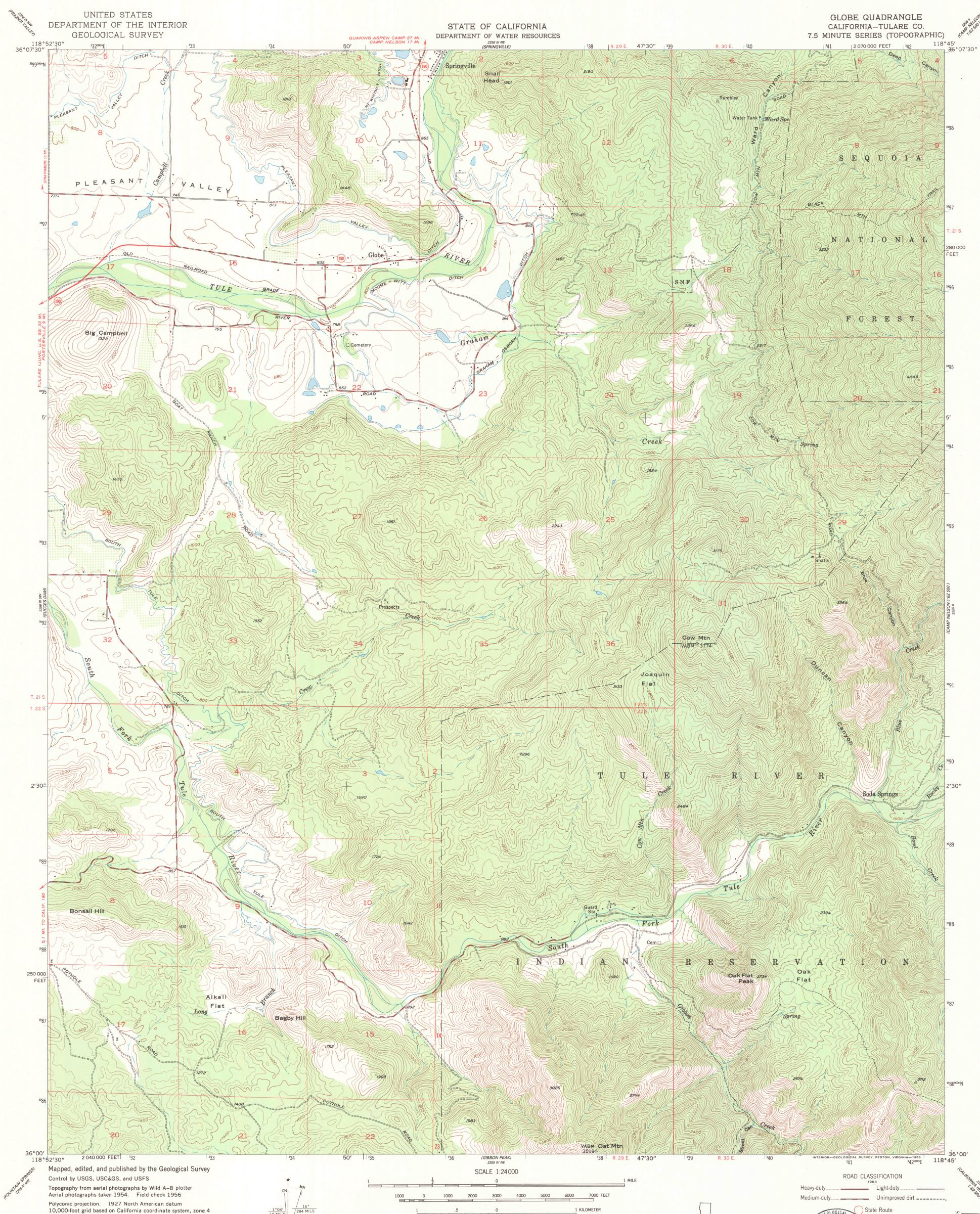
10,000-foot grid based on California coordinate system, zone 4 1000-meter Universal Transverse Mercator grid ticks, zone 11, shown in blue To place on the predicted North American Datum 1983 move the projection lines 7 meters north and 85 meters east as shown by dashed corner ticks
