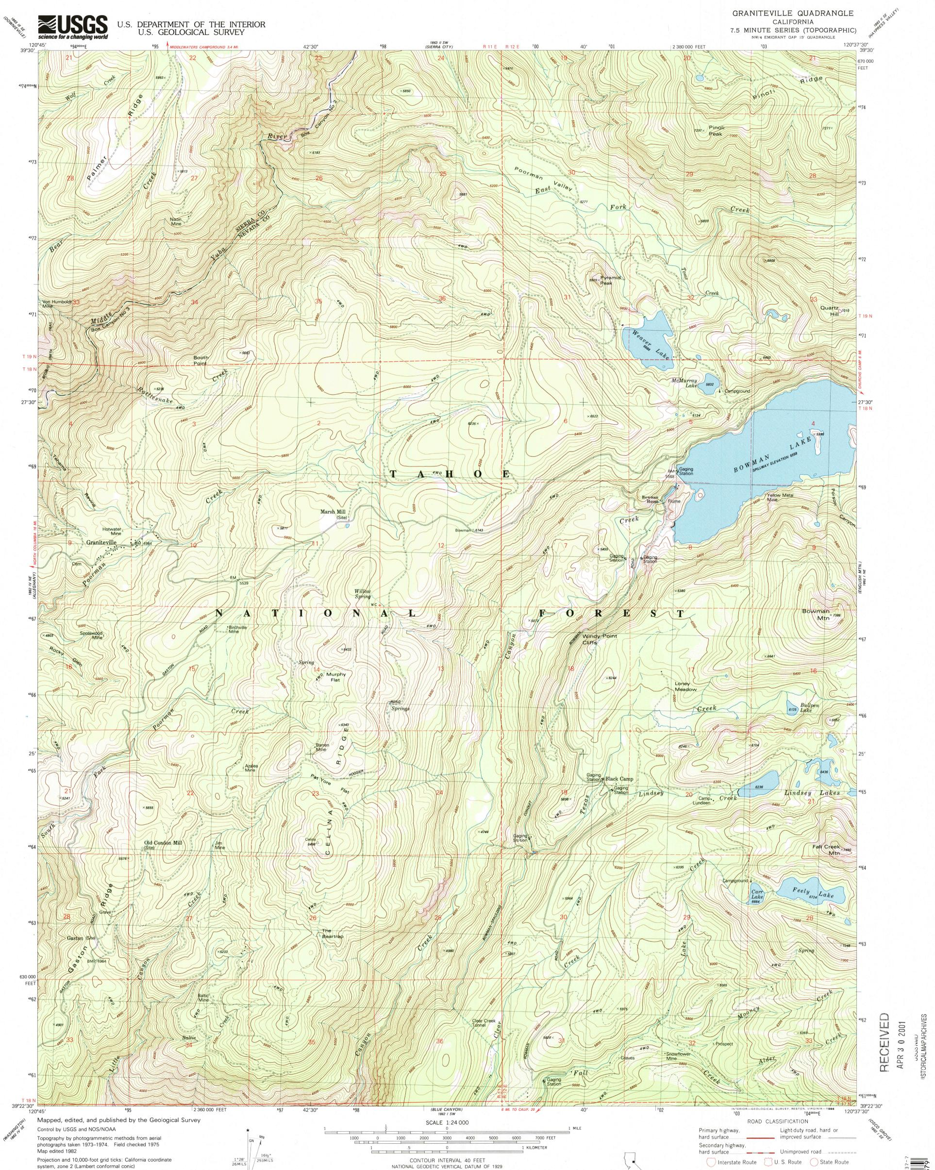
1000-meter Universal Transverse Mercator grid, zone 10 1927 North American Datum To place on the predicted North American Datum 1983 move the projection lines 15 meters north and 89 meters east as shown by dashed corner ticks
