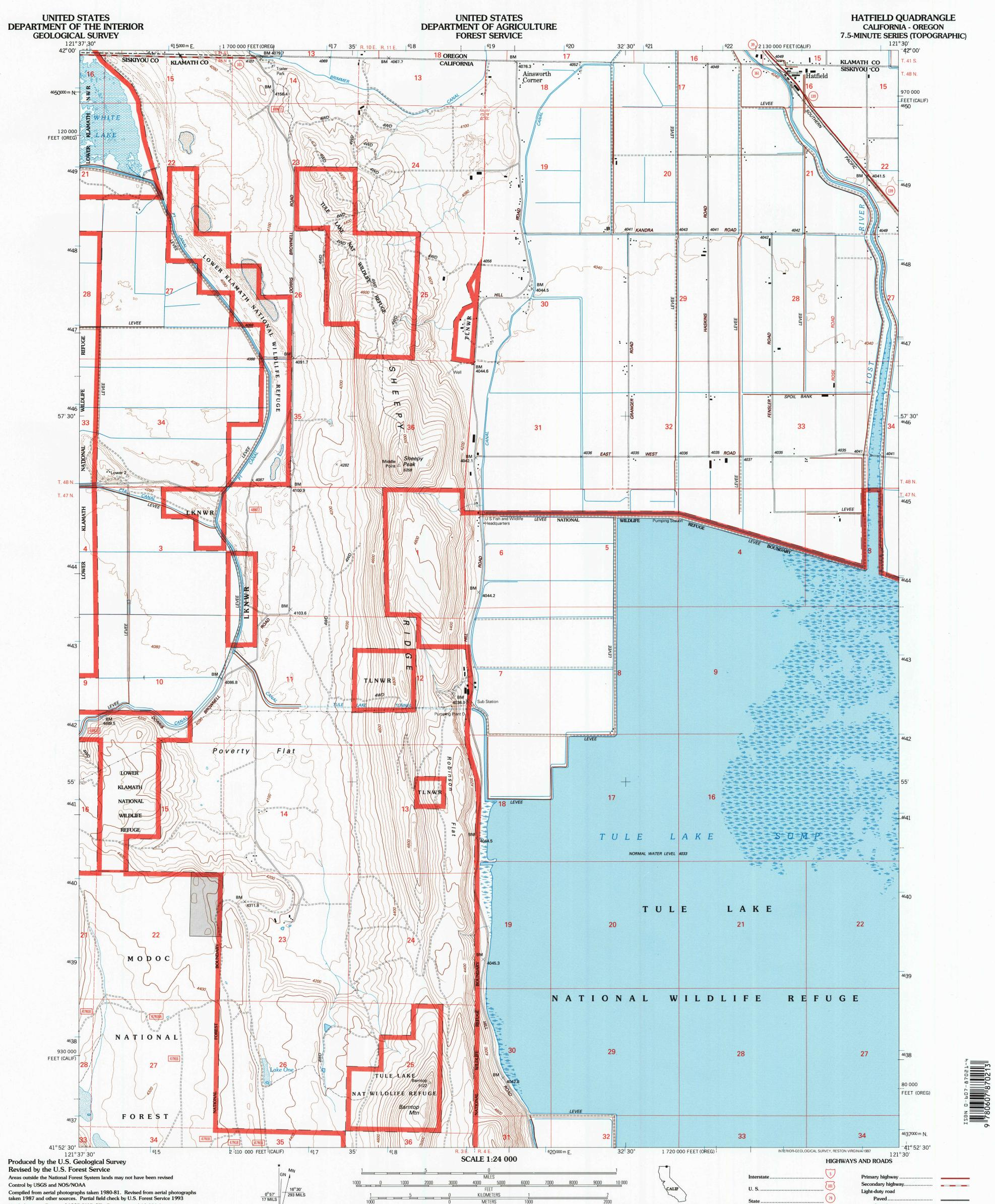
North American Datum of 1927 (NAD 27). Projection and 10 000-foot ticks: California coordinate system, zone 1, and Oregon coordinate system, south zone (Lambert conformal conic) Blue 1000-meter Universal Transverse Mercator ticks, zone 10
