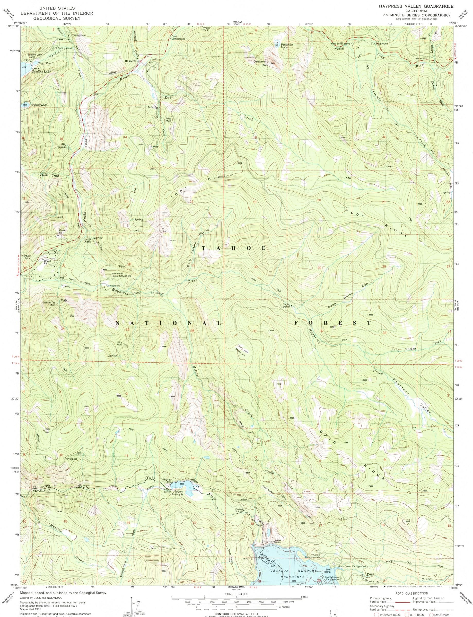
Projection and 10,000-foot grid ticks: California coordinate system, zone 2 (Lambert conformal conic) 1000-meter Universal Transverse Mercator grid, zone 10 1927 North American Datum To place on the predicted North American Datum 1983 move the projection lines 15 meters north and 89 meters east as shown by dashed corner ticks There may be private inholdings within the boundaries of the National or State reservations shown on this map
