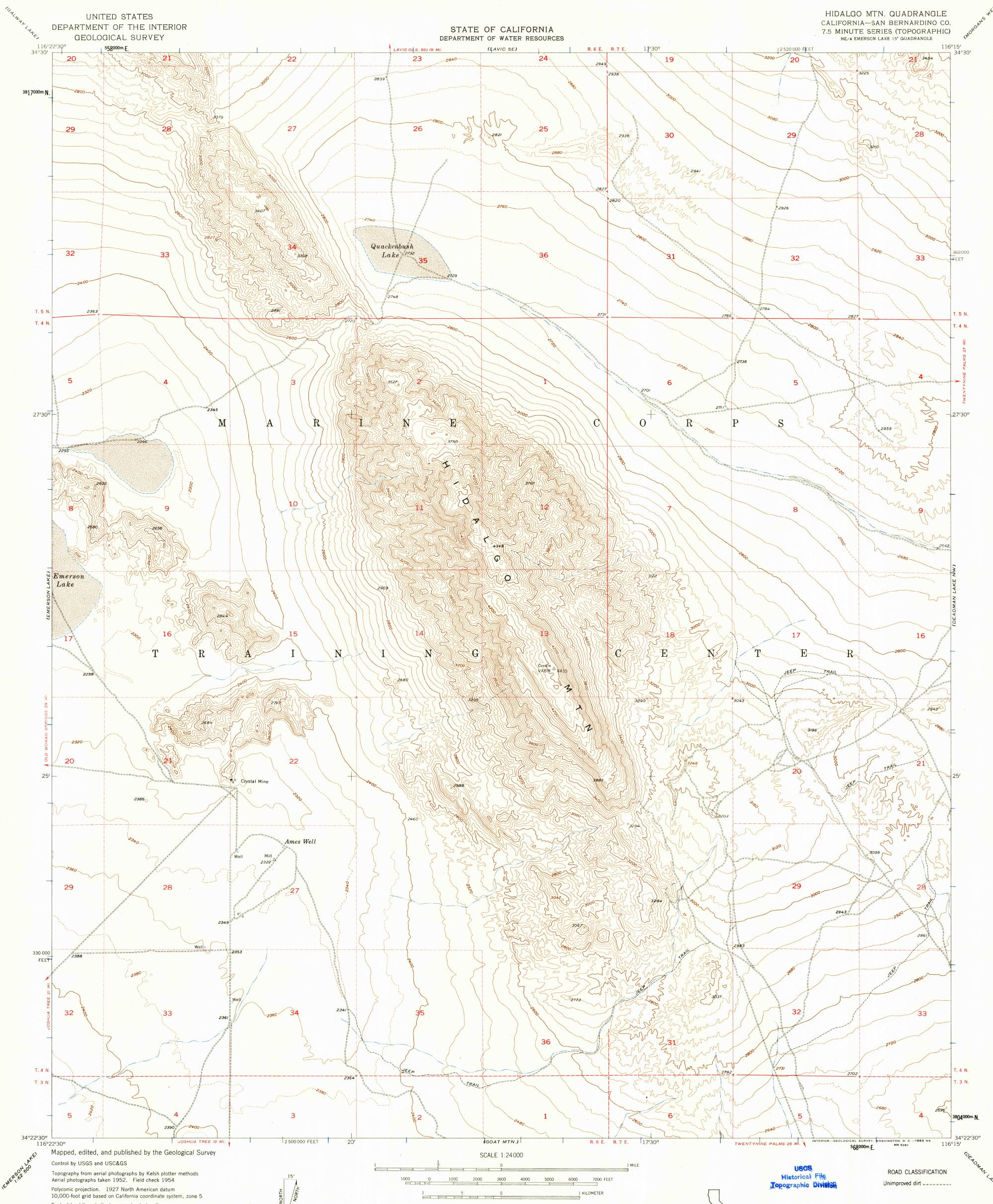
Polyconic projection. 1927 North American datum 10,000-foot grid based on California coordinate system, zone 5 Dashed land lines indicate approximate locations Unchecked elevations are shown in brown 1000-meter Universal Transverse Mercator grid ticks,
