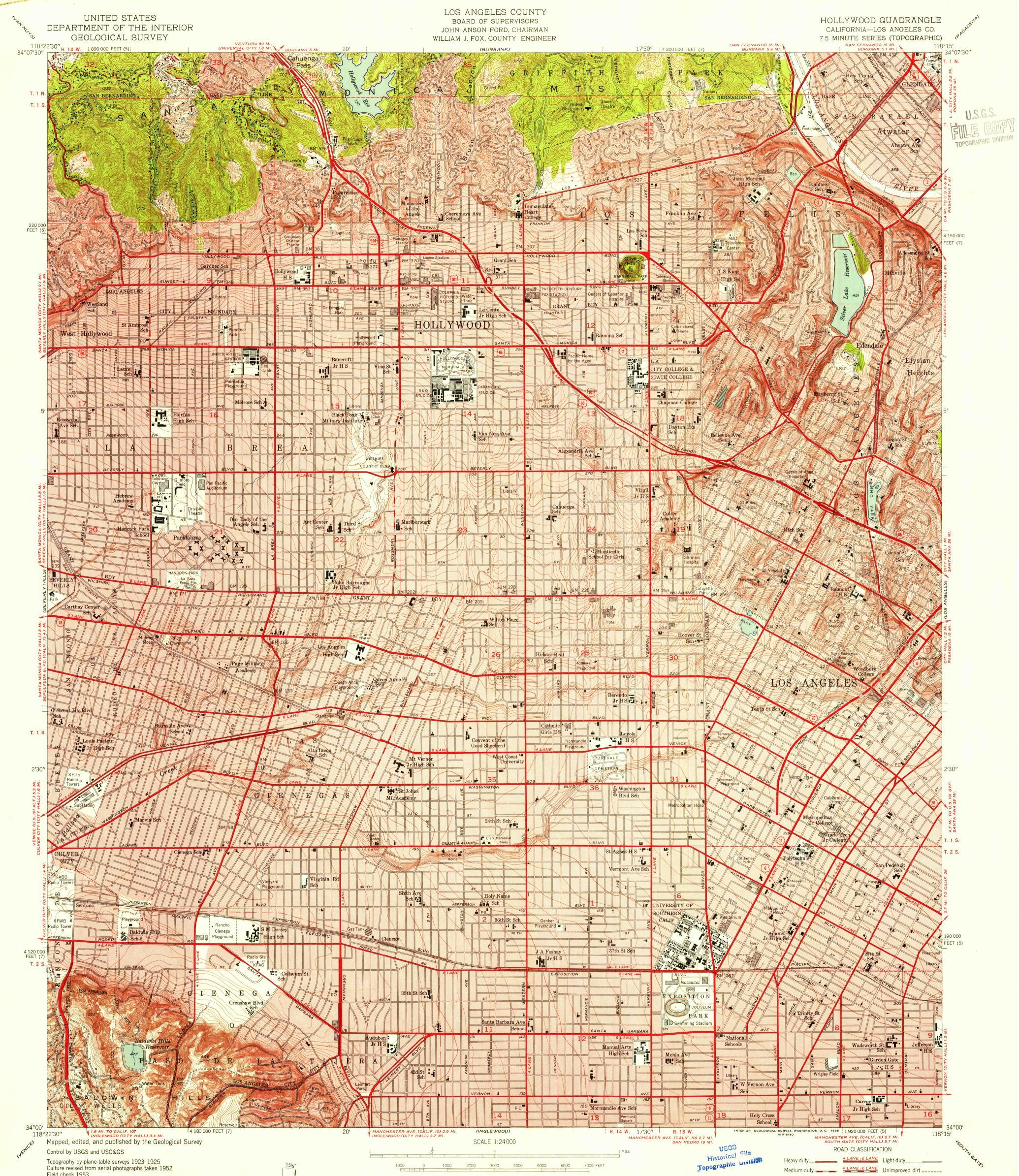
Polyconic projection. 1927 North American datum 10,000-foot grids based on California coordinate system, zones 5 and 7
