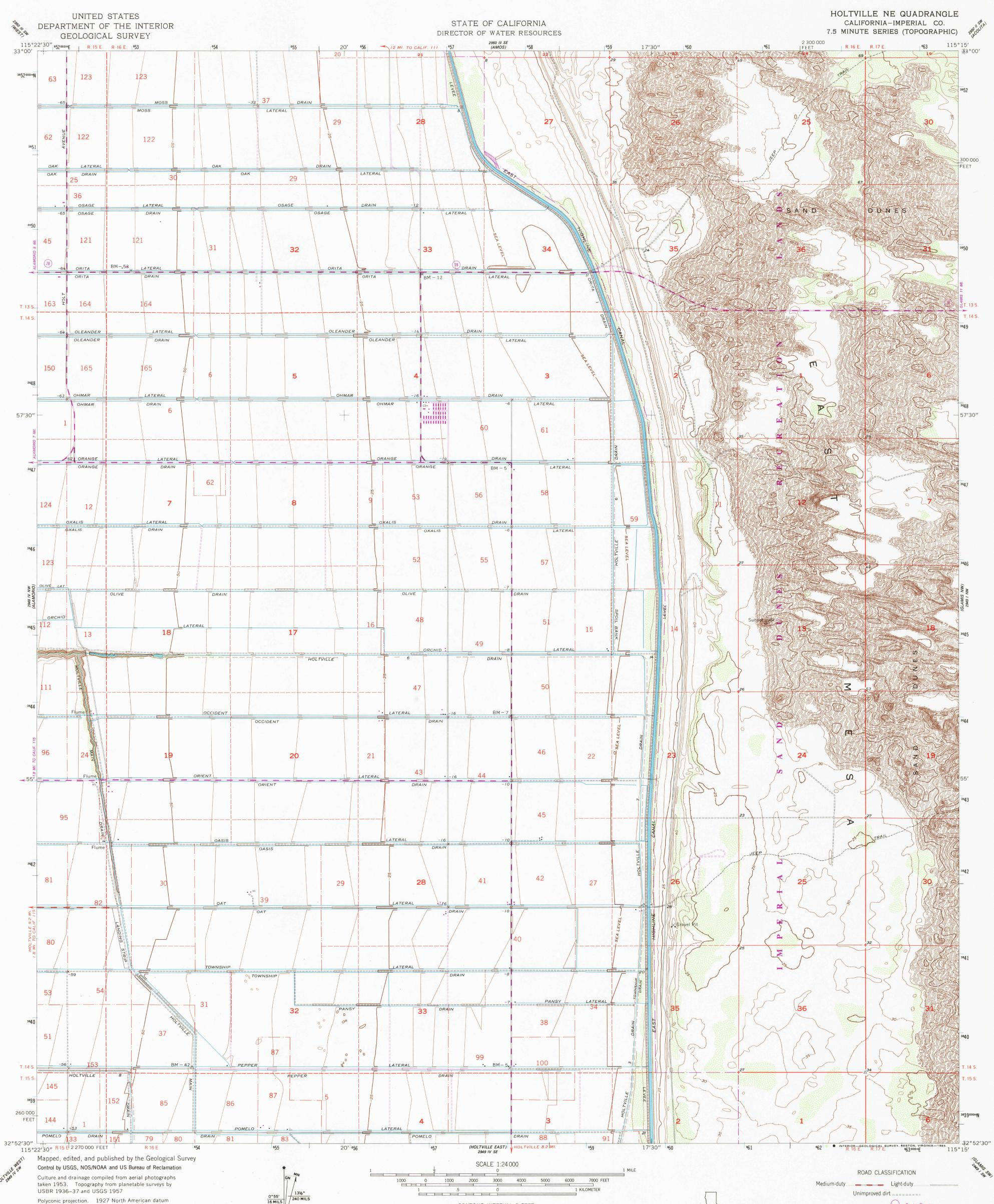
Polyconic projection. 1927 North American datum 10,000-foot grid based on California coordinate system, zone 6 1000-meter Universal Transverse Mercator grid ticks, zone 11, shown in blue To place on the predicted North American Datum 1983, move the projection lines 4 meters south and 75 meters east as shown by dashed corner ticks There may be private inholdings within the boundaries of the National or State reservations shown on this map
