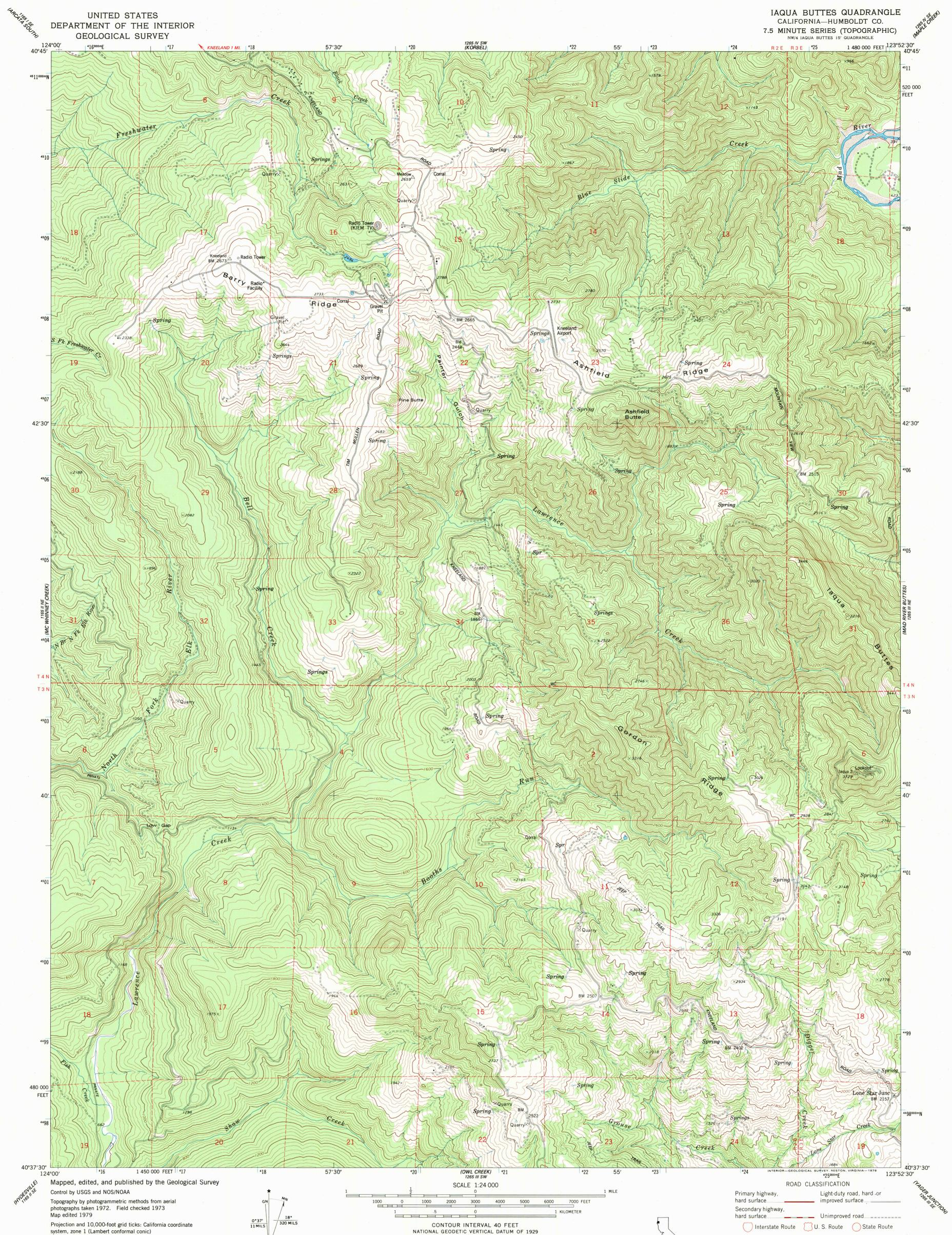
1000-meter Universal Transverse Mercator grid ticks, zone 10, shown in blue. 1927 North American Datum To place on the predicted North American Datum 1983 move the projection lines 20 meters north and 96 meters east as shown by dashed corner ticks
