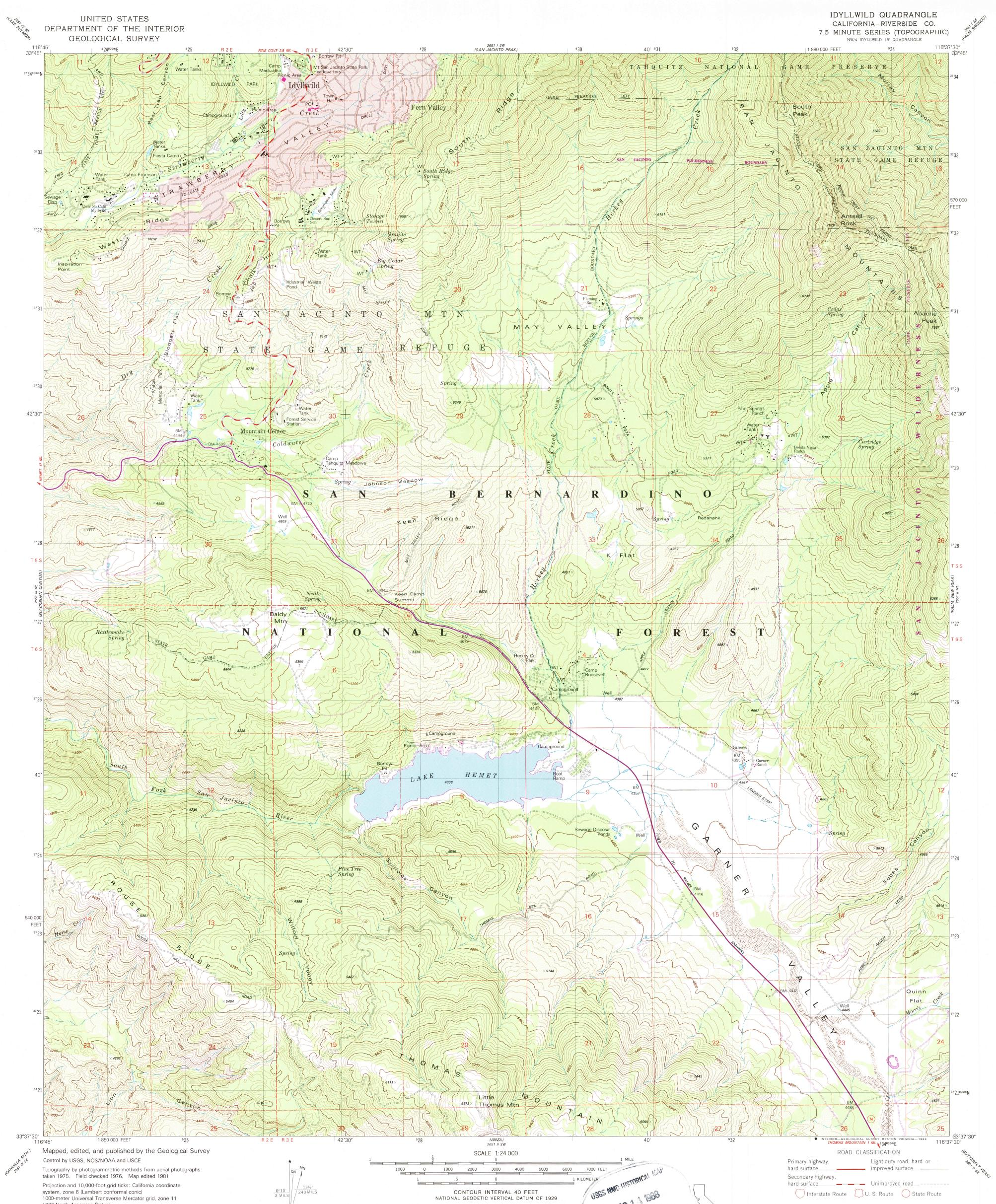
system, zone 6 (Lambert conformal conic) 1000-meter Universal Transverse Mercator grid, zone 11 1927 North American Datum To place on the predicted North American Datum 1983 move the projection lines 80 meters east as shown by dashed corner ticks
