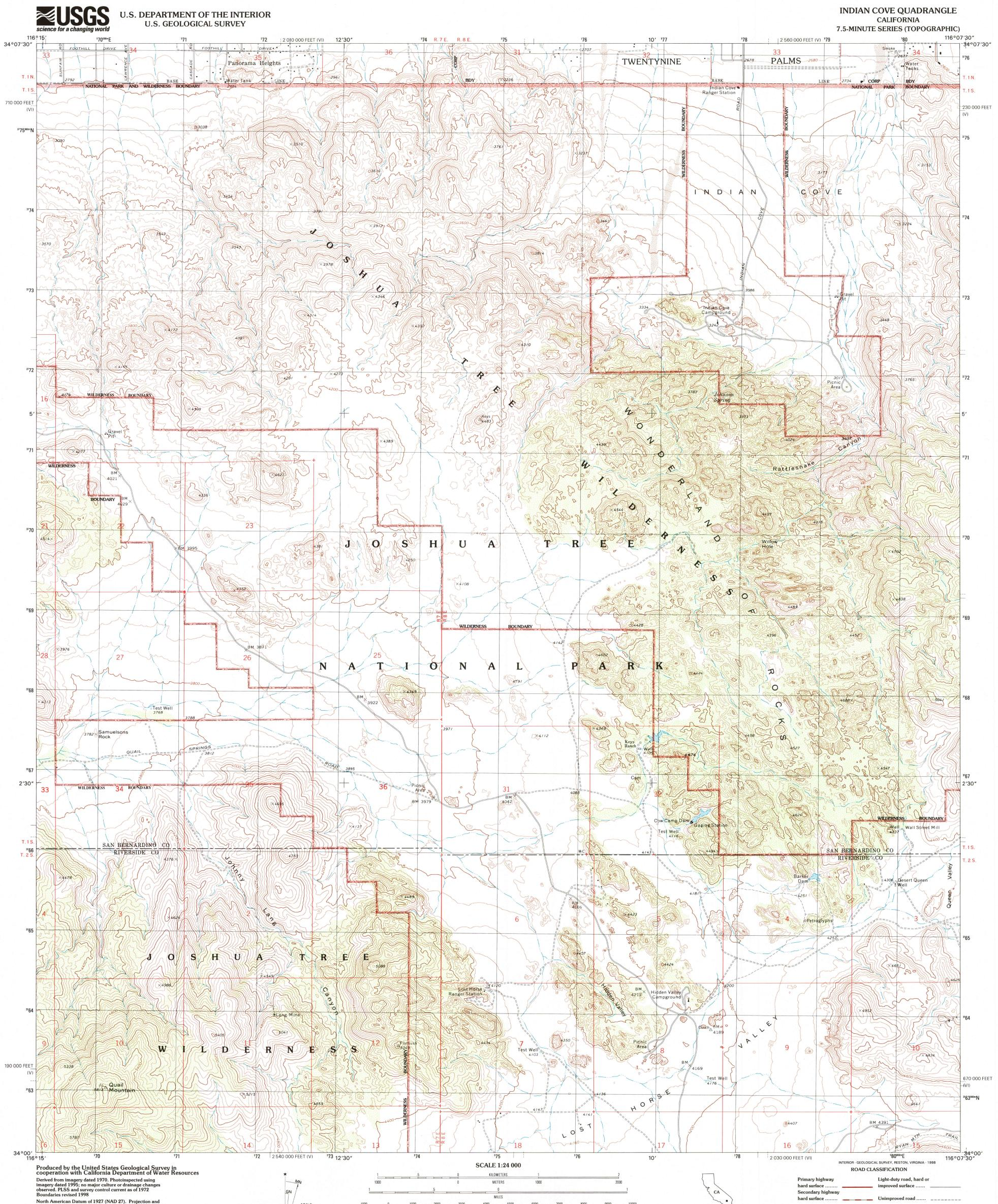
North American Datum of 1927 (NAD 27). Projection and 1000-meter grid: Universal Transverse Mercator, zone 11 10 000-foot ticks: California Coordinate System of 1927 (zones 5 and 6)
