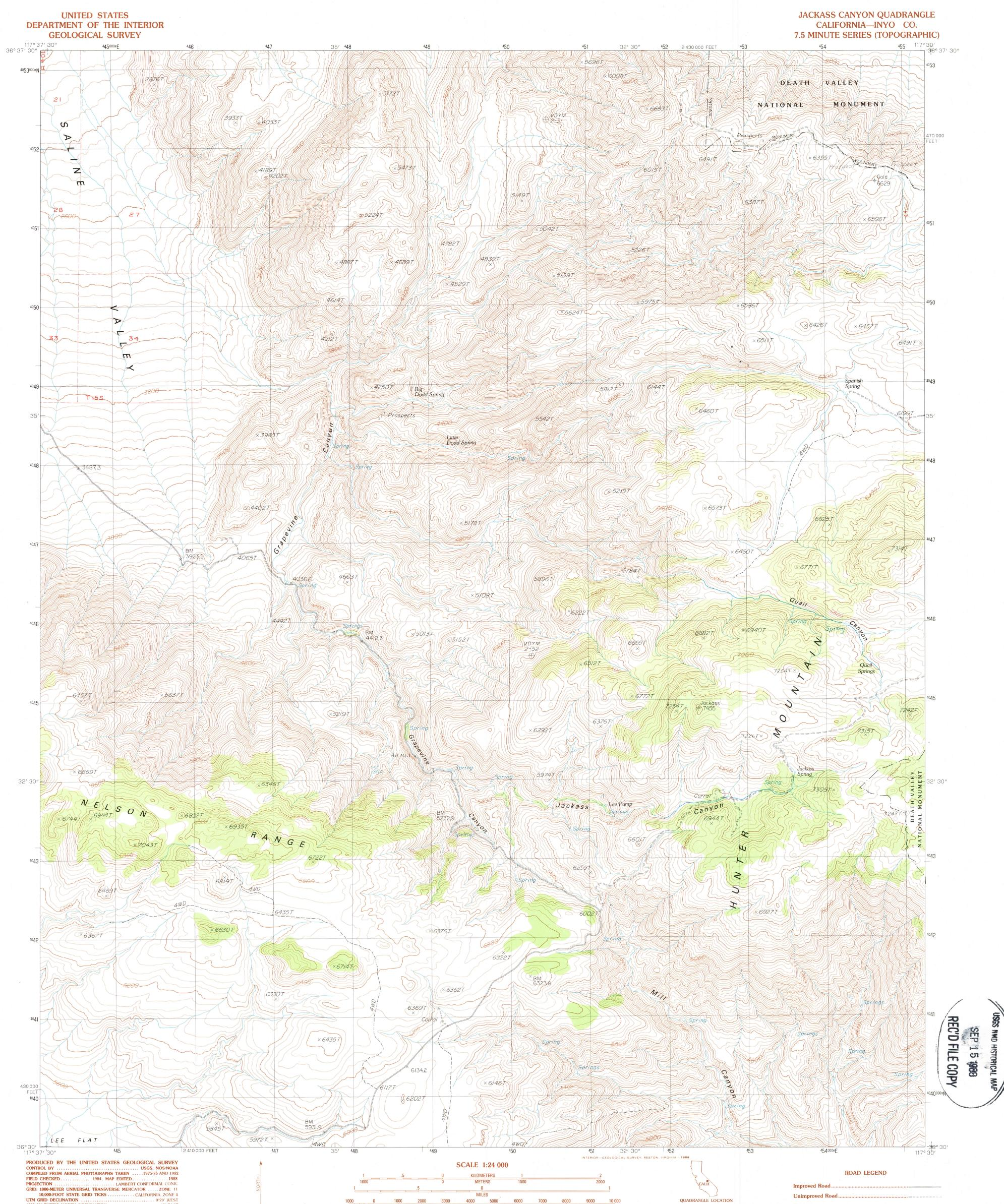
1980 MAGNETIC NORTH DECLINATION ..... ....15° EAST VERTICAL DATUM ... NATIONAL GEODETIC VERTICAL DATUM OF 1929 HORIZONTAL DATUM ...... 1927 NORTH AMERICAN DATUM To place on the predicted North American Datum of 1983, move the projection lines as shown by dashed corner ticks ( 8 meters north / 81 meters east ) There may be private inholdings within the boundaries of any Federal and State Reservations shown on this map
