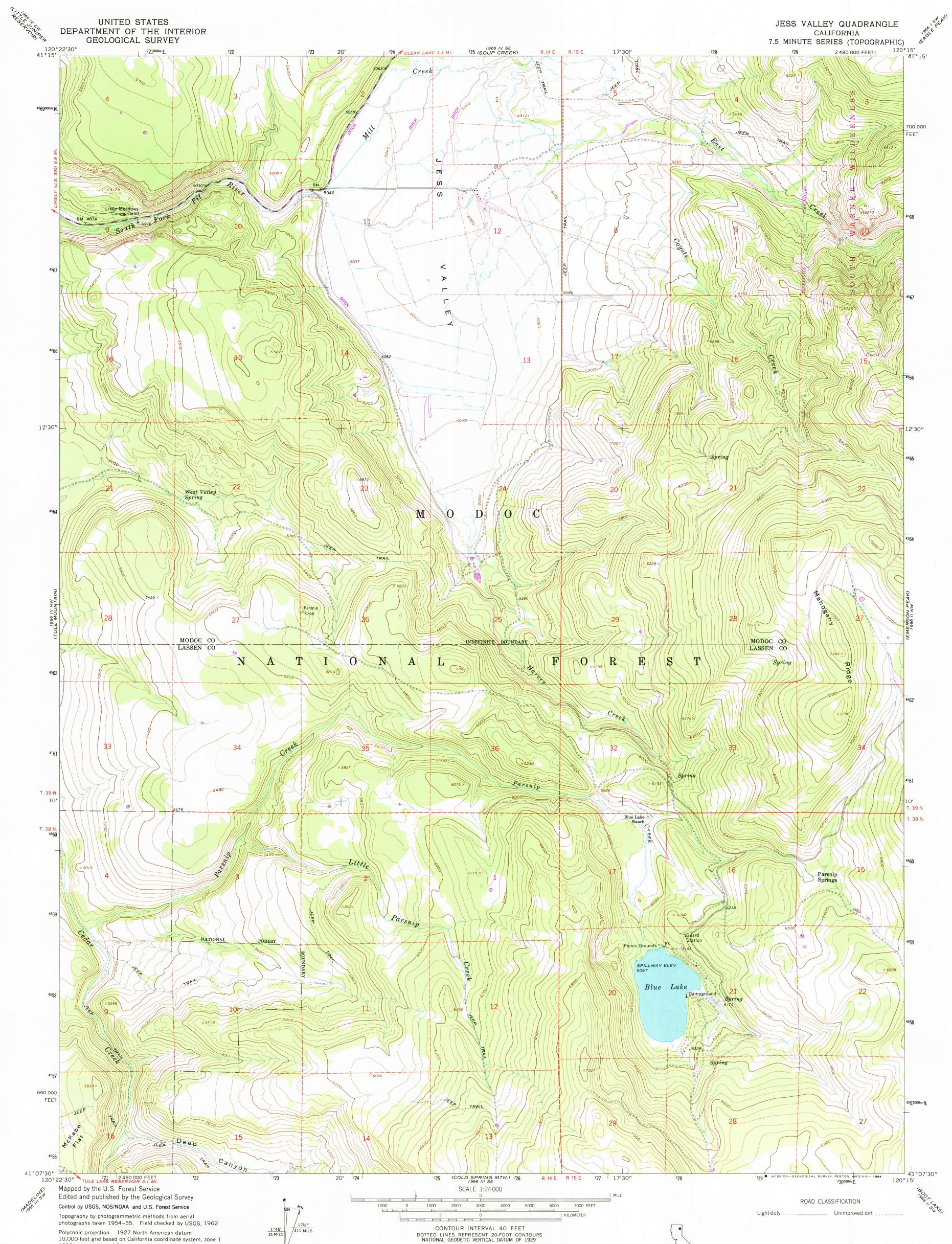
Polyconic projection. 1927 North American datum 10,000-foot grid based on California coordinate system, zone 1 1000-meter Universal Transverse Mercator grid ticks, zone 10, shown in blue Fine red dashed lines indicate selected fence lines To place on the predicted North American Datum 1983 move the projection lines 17 meters north and 88 meters east as shown by dashed corner ticks There may be private inholdings within the boundaries of the National or State reservations shown on this map
