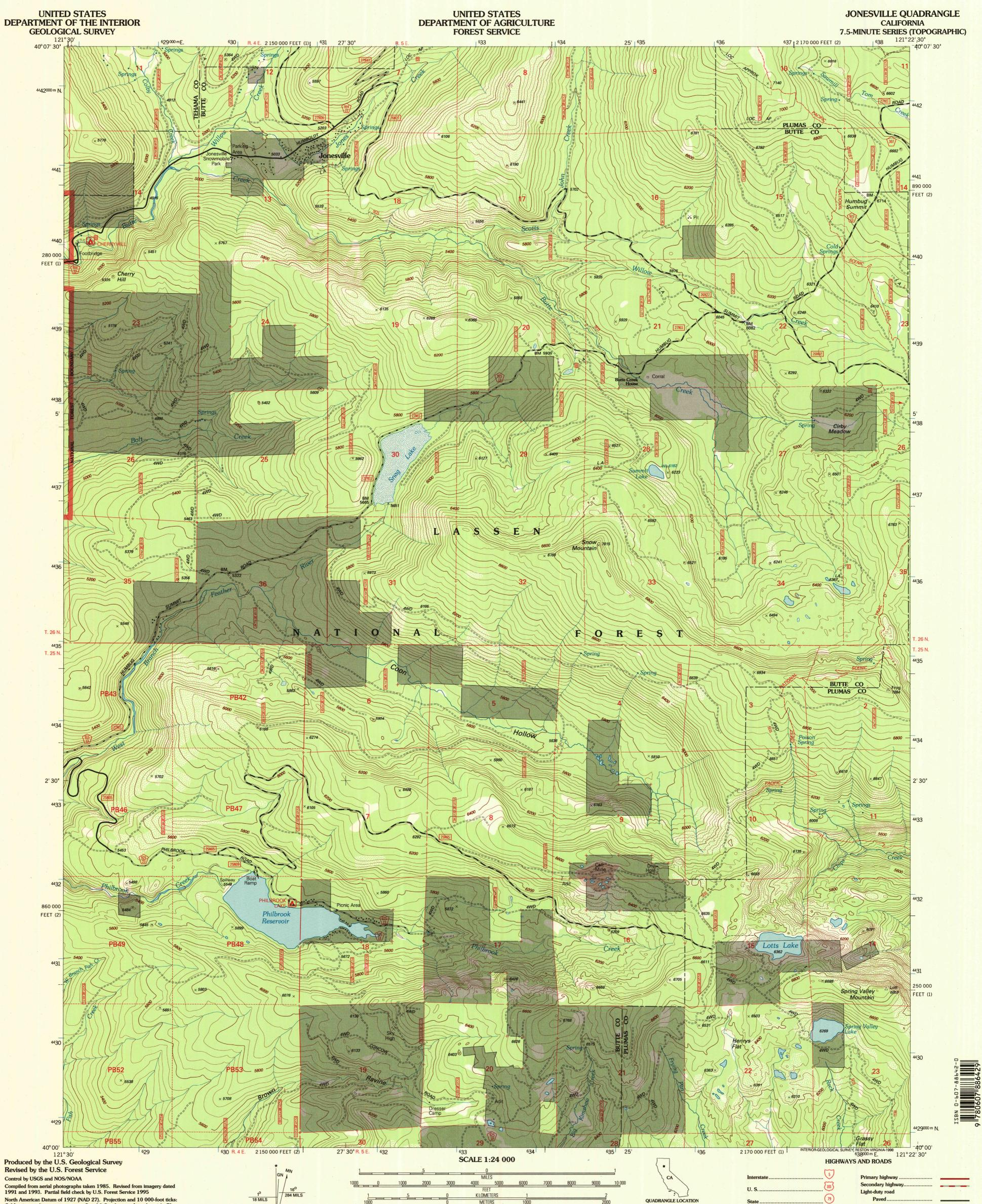
California coordinate system, zones 2 and 1 (Lambert conformal conic). Blue 1000-meter Universal Transverse Mercator ticks, zone 10
