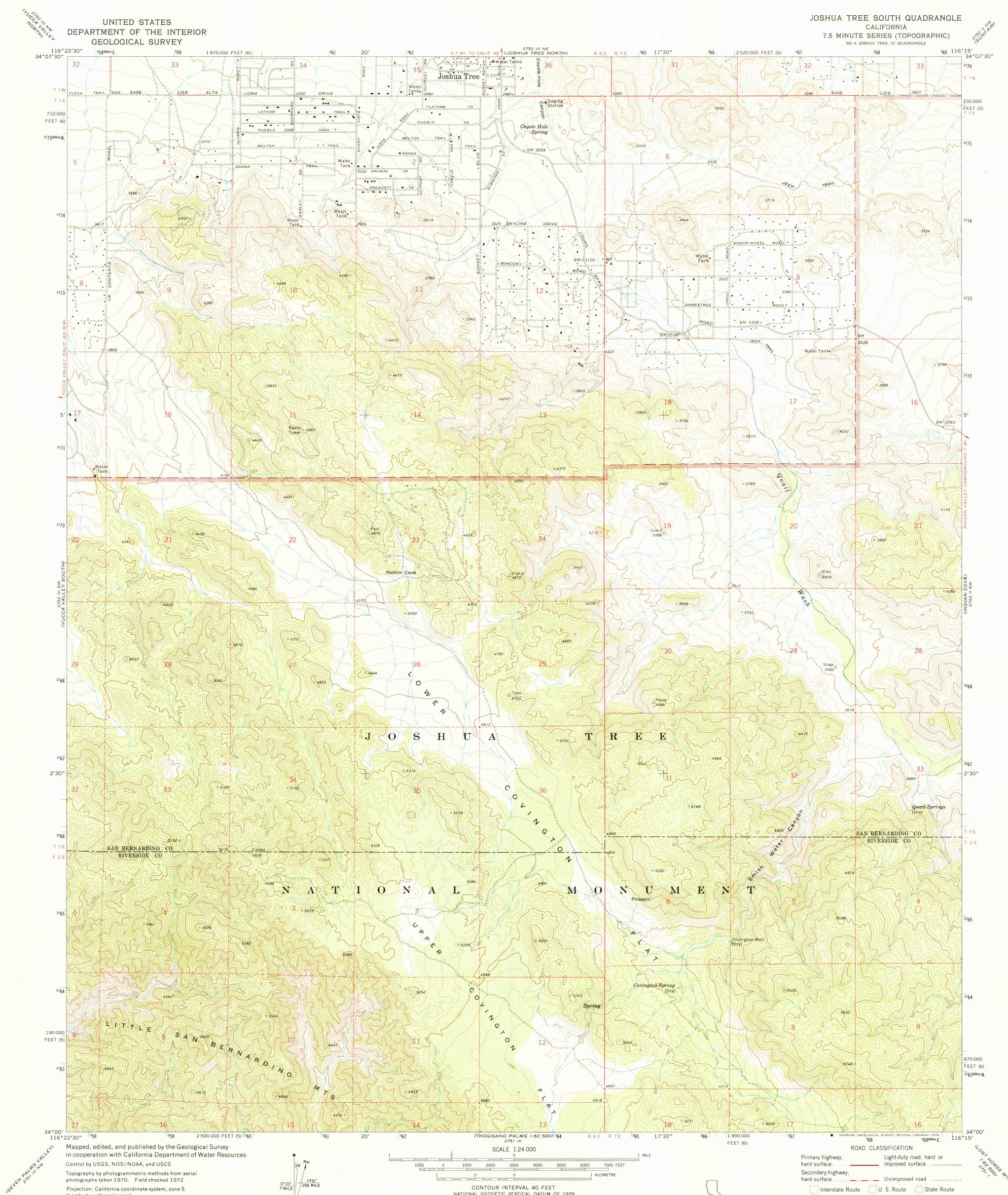
Projection: California coordinate system, zone 5 (Lambert conformal conic) 10,000-foot grid ticks based on California coordinate system, zones 5 and 6 1000-metre Universal Transverse Mercator grid ticks, zone 11, shown in blue. 1927 North American datum Where omitted, land lines have not been established
