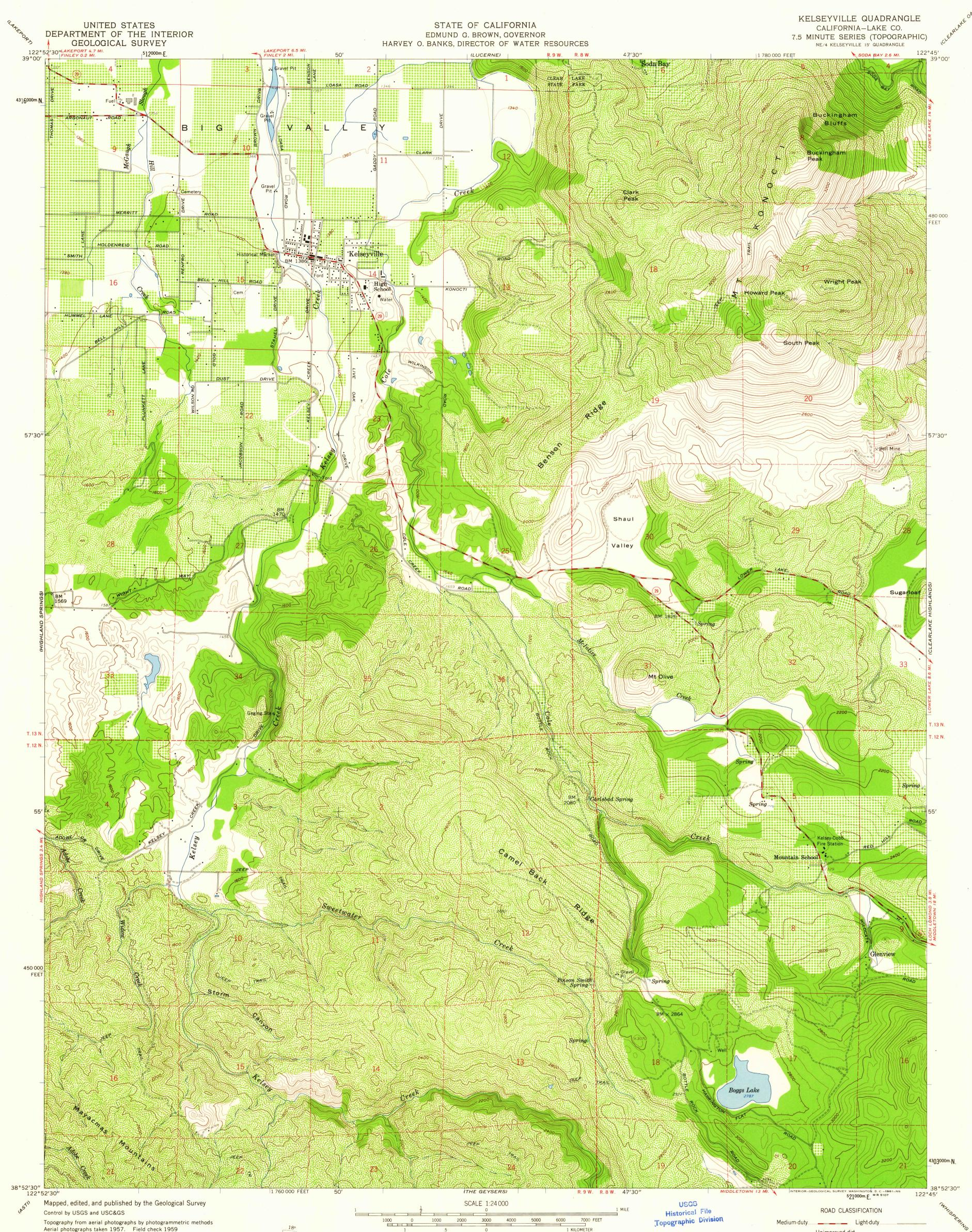
Aerial photographs taken 1957. Field check 1959 Polyconic projection. 1927 North American datum 10,000-foot grid based on California coordinate system, zone 2 1000-meter Universal Transverse Mercator grid ticks, zone 10, shown in blue Dashed land lines indicate approximate locations
