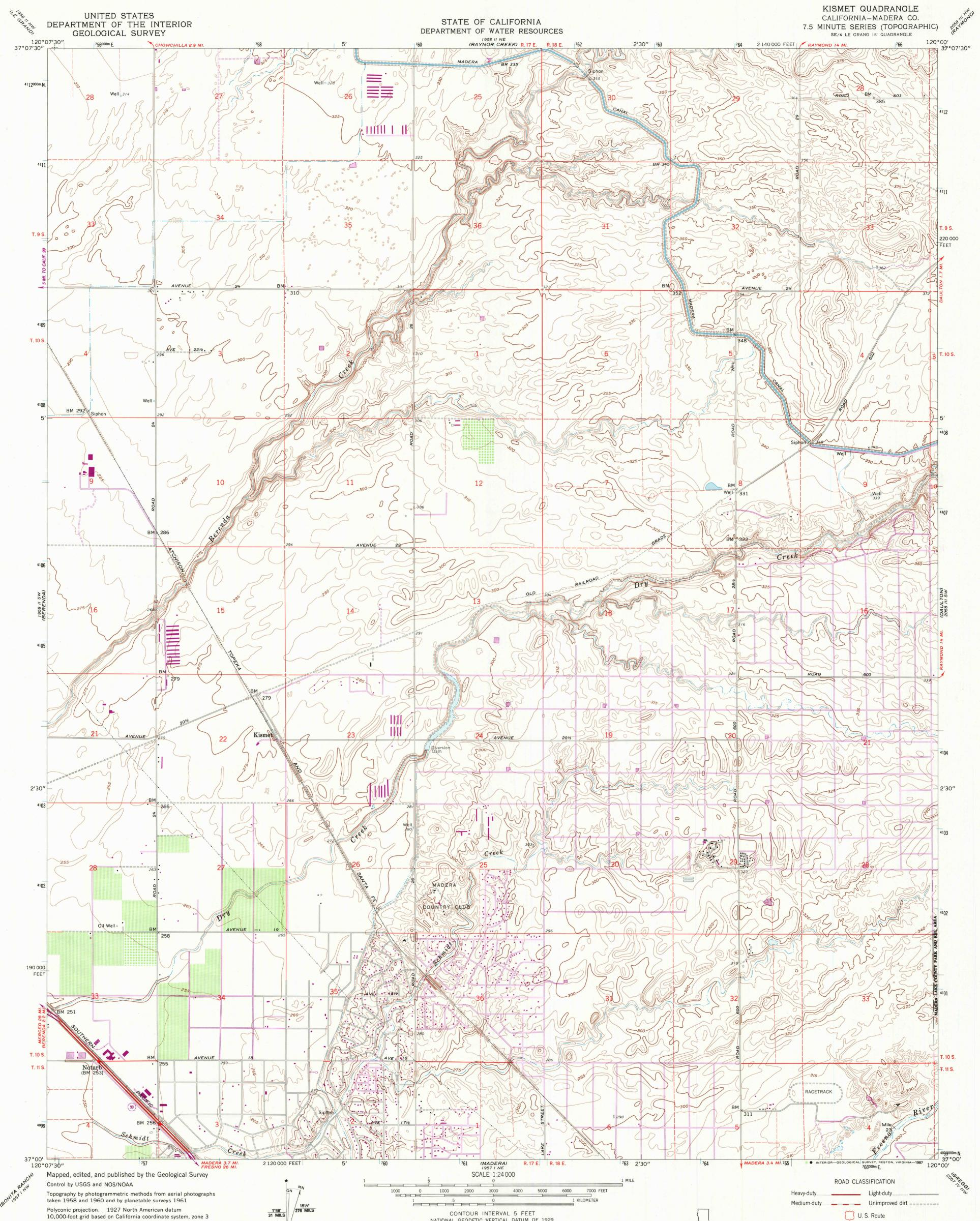
10,000-foot grid based on California coordinate system, zone 3 1000-meter Universal Transverse Mercator grid ticks, zone 10, shown in blue To place on the predicted North American Datum 1983 move the projection lines 10 meters north and 89 meters east as shown by dashed corner ticks
