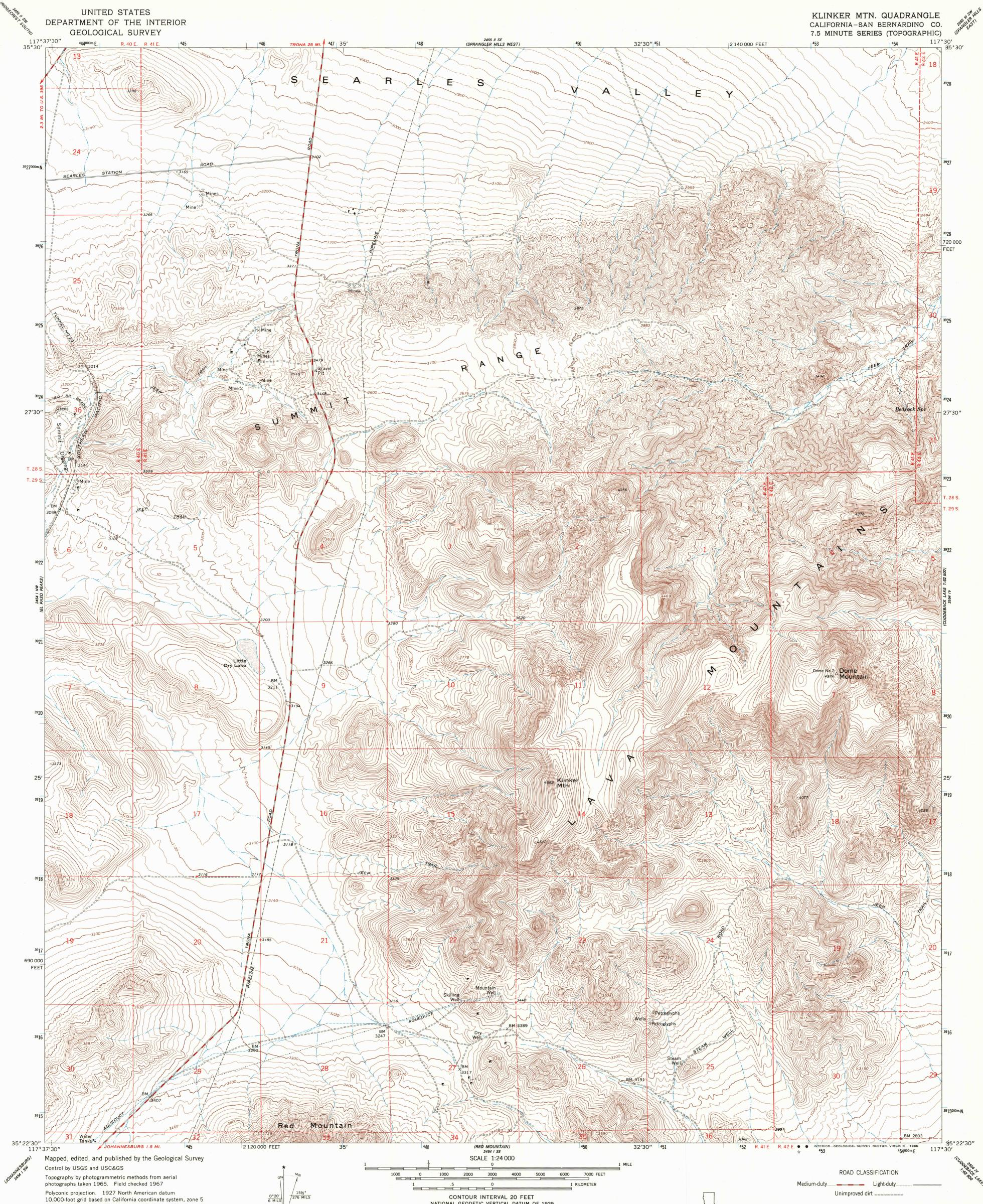
10,000-foot grid based on California coordinate system, zone 5 1000-meter Universal Transverse Mercator grid ticks, zone 11, shown in blue To place on the predicted North American Datum 1983, move the projection lines 6 meters north and 82 meters east as shown by dashed corner ticks
