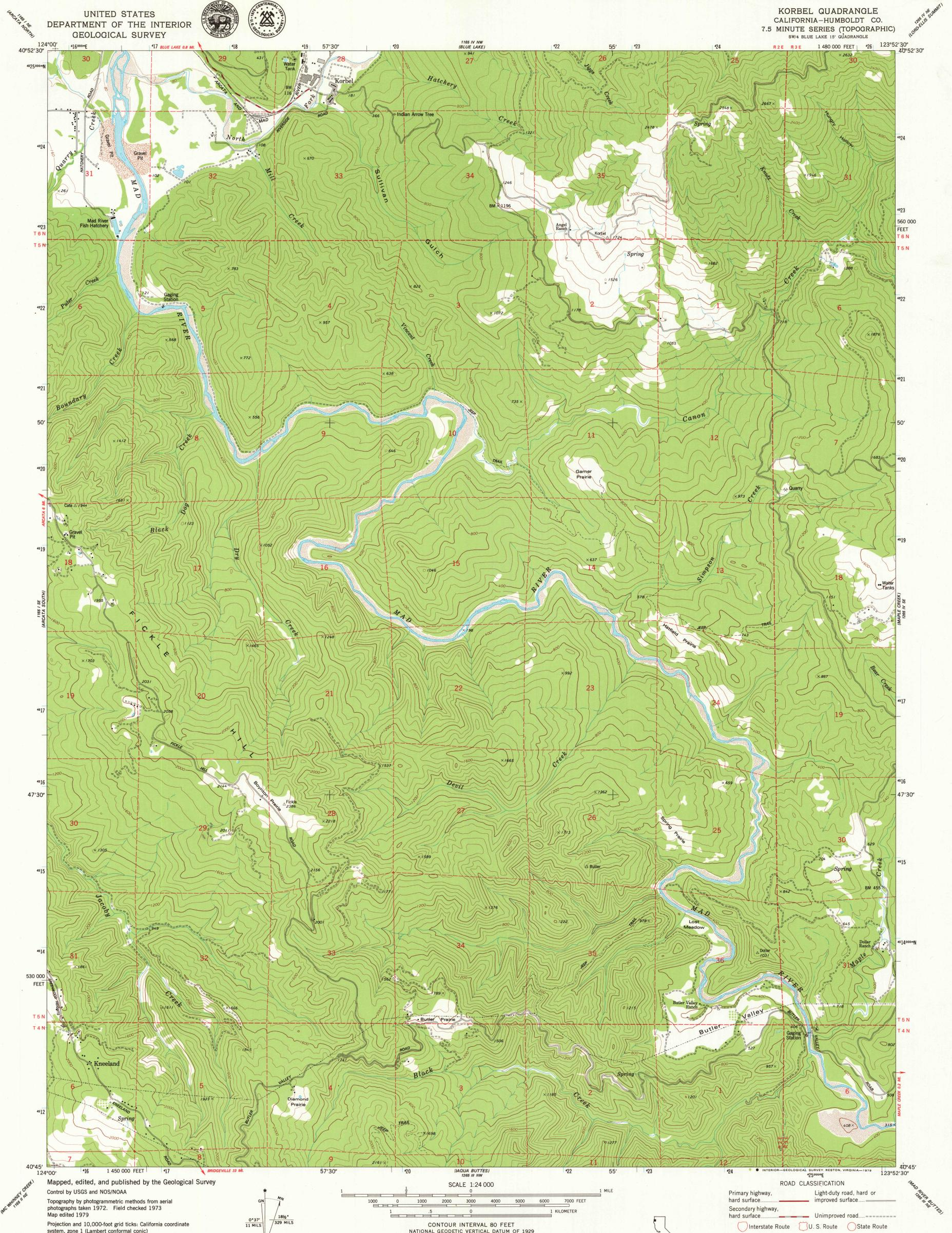
system, zone 1 (Lambert conformal conic) 1000-meter Universal Transverse Mercator grid ticks, zone 10, shown in blue. 1927 North American datum To place on the predicted North American Datum 1983 move the projection lines 20 meters north and 96 meters east as shown by dashed corner ticks
