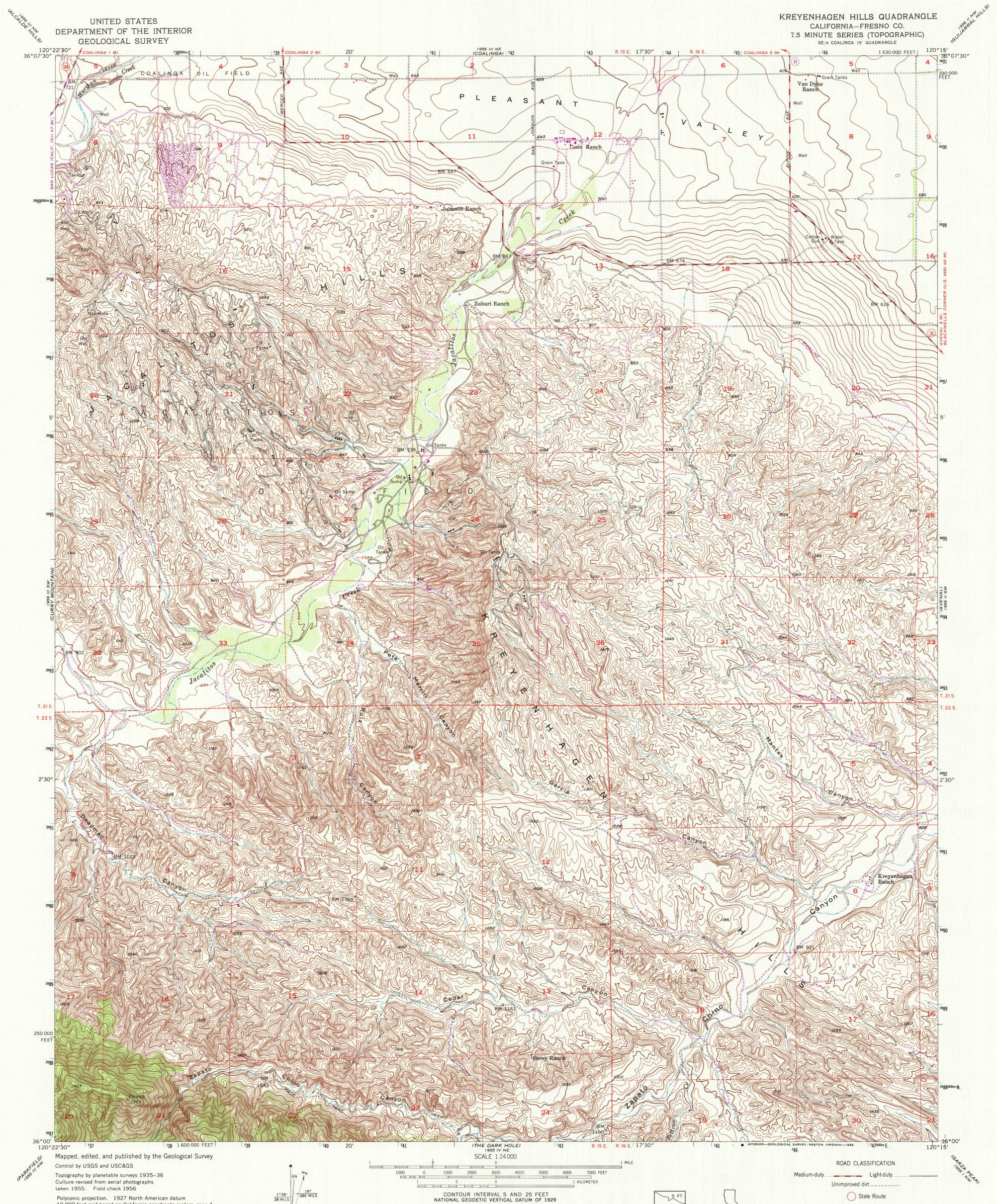
Polyconic projection. 1927 North American datum 10,000-foot grid based on California coordinate system, zone 4 1000-meter Universal Transverse Mercator grid ticks, zone 10, shown in blue To place on the predicted North American Datum 1983 move the projection lines 9 meters north and 91 meters east as shown by dashed corner ticks Revisions shown in purple compiled from aerial photographs taken 1971. This information not field checked
