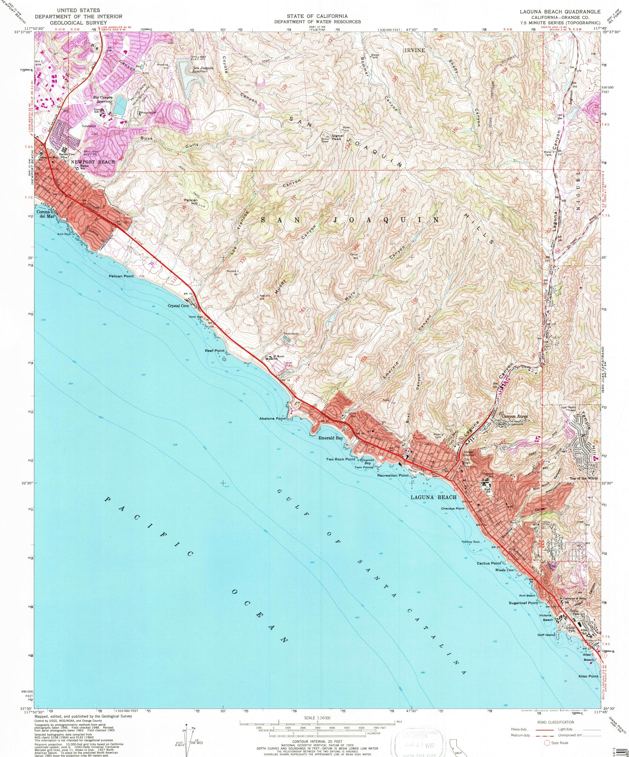
Polyconic projection. 10,000-foot grid ticks based on California coordinate system, zone 6. 1000-meter Universal Transverse Mercator grid ticks, zone 11, shown in blue. 1927 North American Datum. To place on the predicted North American Datum 1983 move the projection lines 84 meters east as shown by dashed corner ticks
