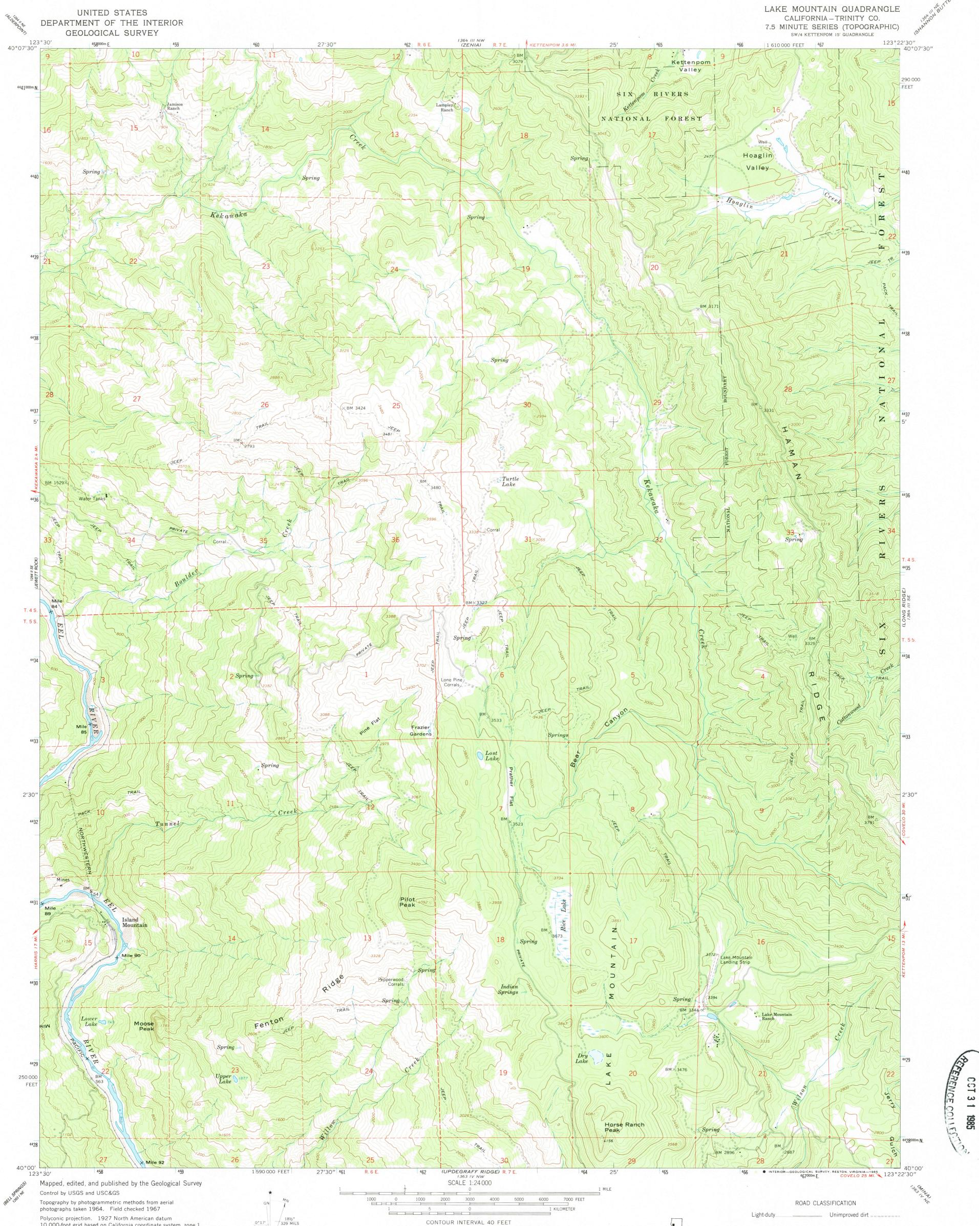
10,000-foot grid based on California coordinate system, zone 1 1000-meter Universal Transverse Mercator grid ticks, zone 10, shown in blue To place on the predicted North American Datum 1983 move the projection lines 19 meters north and 95 meters east as shown by dashed corner ticks DOTTED LINES CROSSING RIVERS REPRESENT 20-FOOT CONTOURS NATIONAL GEODETIC VERTICAL DATUM OF 1929
