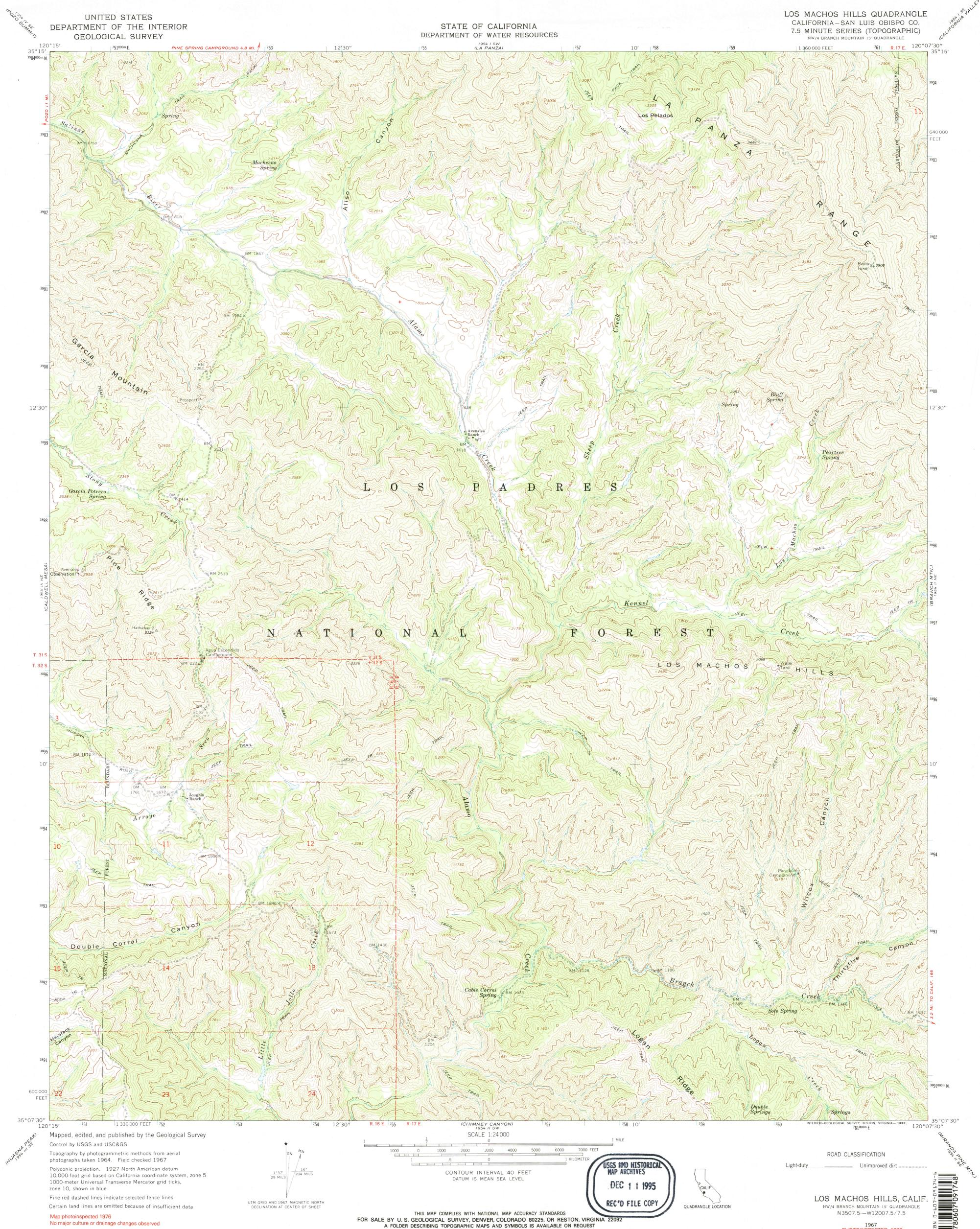
10,000-foot grid based on California coordinate system, zone 5 1000-meter Universal Transverse Mercator grid ticks, zone 10, shown in blue
