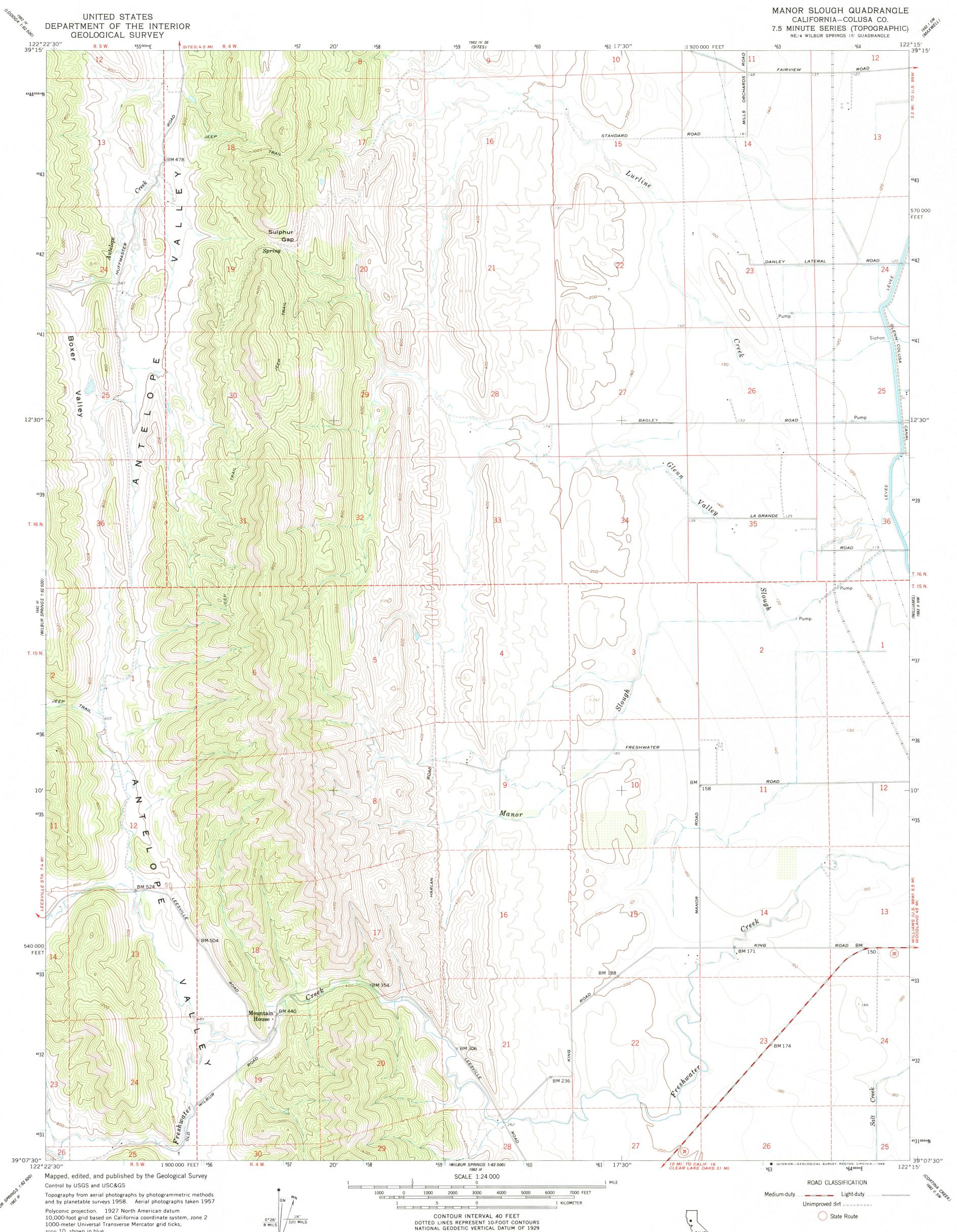
1000-meter Universal Transverse Mercator grid ticks, zone 10, shown in blue To place on the predicted North American Datum 1983 move the projection lines 16 meters north and 94 meters east as shown by dashed corner ticks
