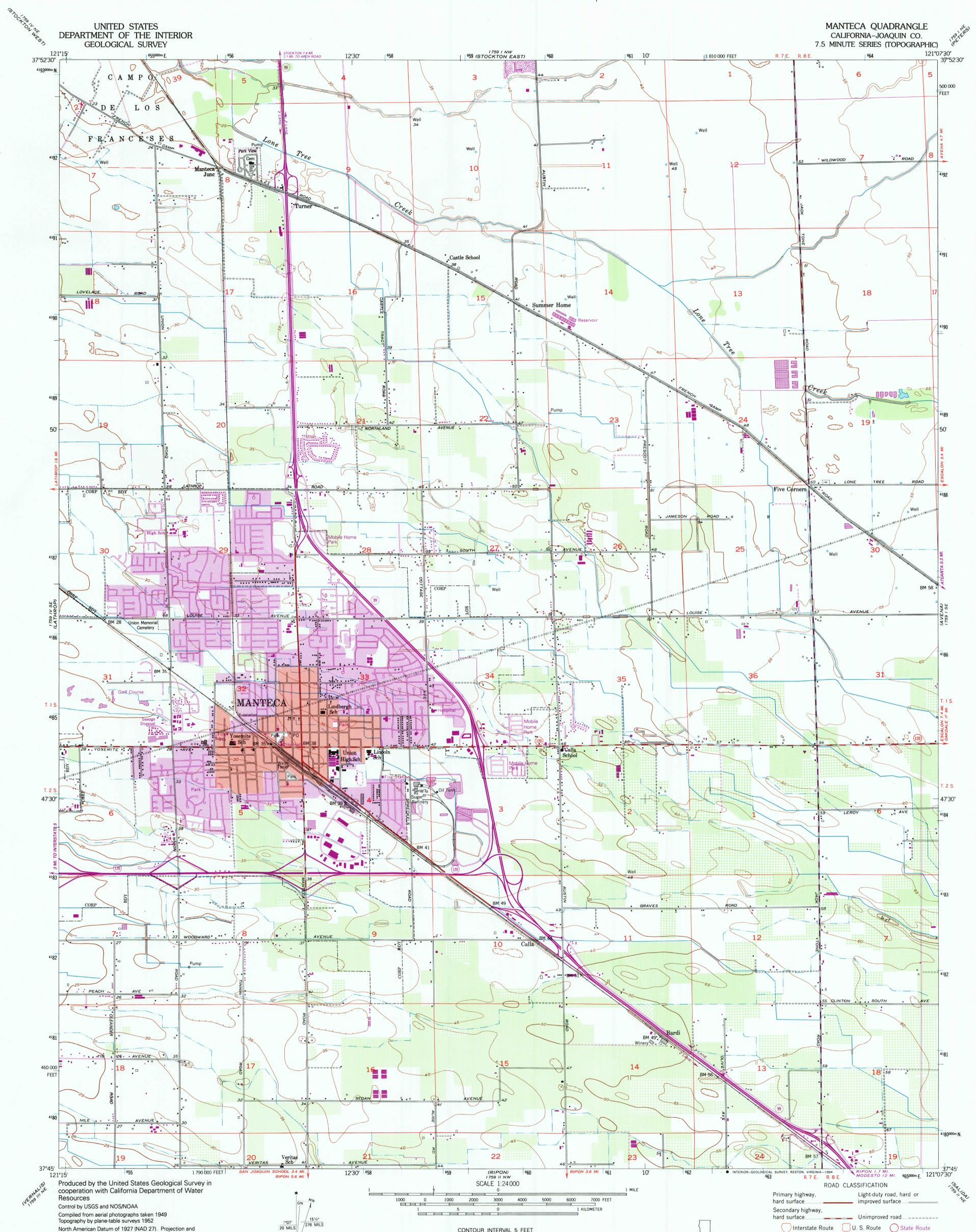
North American Datum of 1927 (NAD 27). Projection and 10000-foot ticks: California Coordinate System, zone 3 (Lambert Conformal Conic) Blue 1000-meter Universal Transverse Mercator ticks, zone 10 North American Datum of 1983 (NAD 83) is shown by dashed corner ticks. The values of the shift between NAD 27 and NAD 83 for 7.5-minute intersections are obtainable from National Geodetic Survey NADCON software
