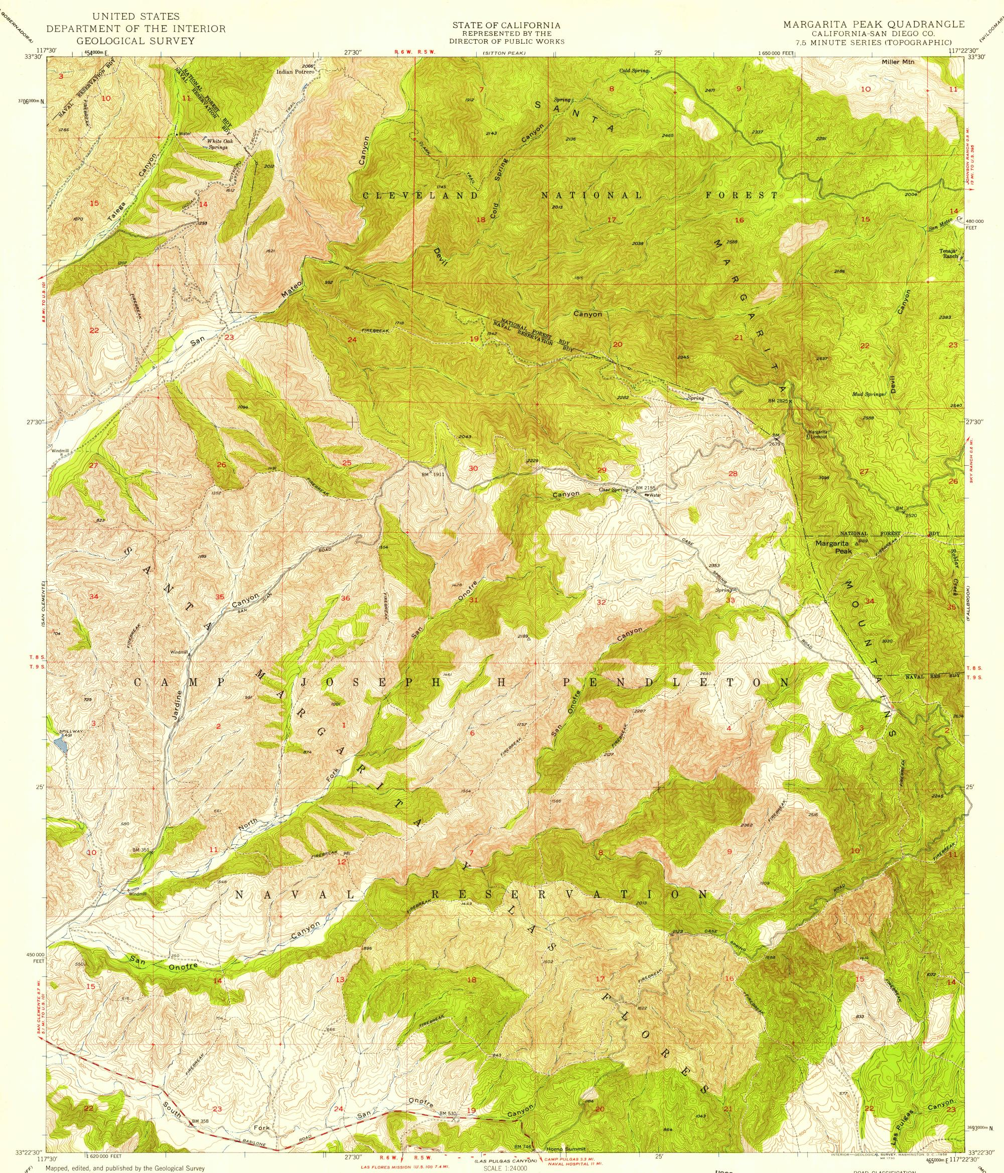
Control by USC&GS, U.S. Army, and U.S. Navy Topography from aerial photographs by multiplex methods Aerial photographs taken 1946. Field check 1949 SCALE 1:24000
