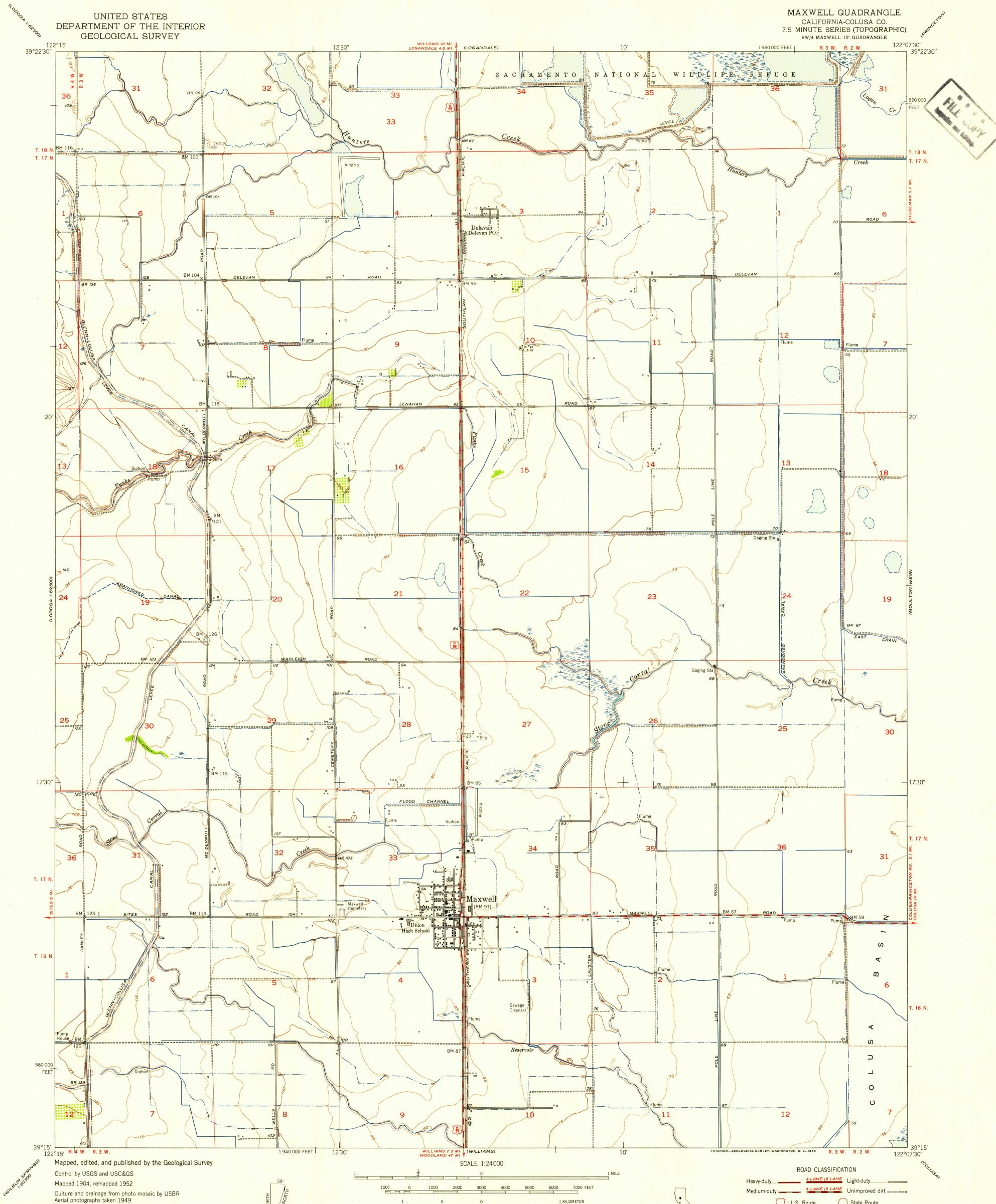
Topography from plane-table surveys by USGS 1952 Polyconic projection. 1927 North American datum 10,000-foot grid based on California coordinate system, zone 2
