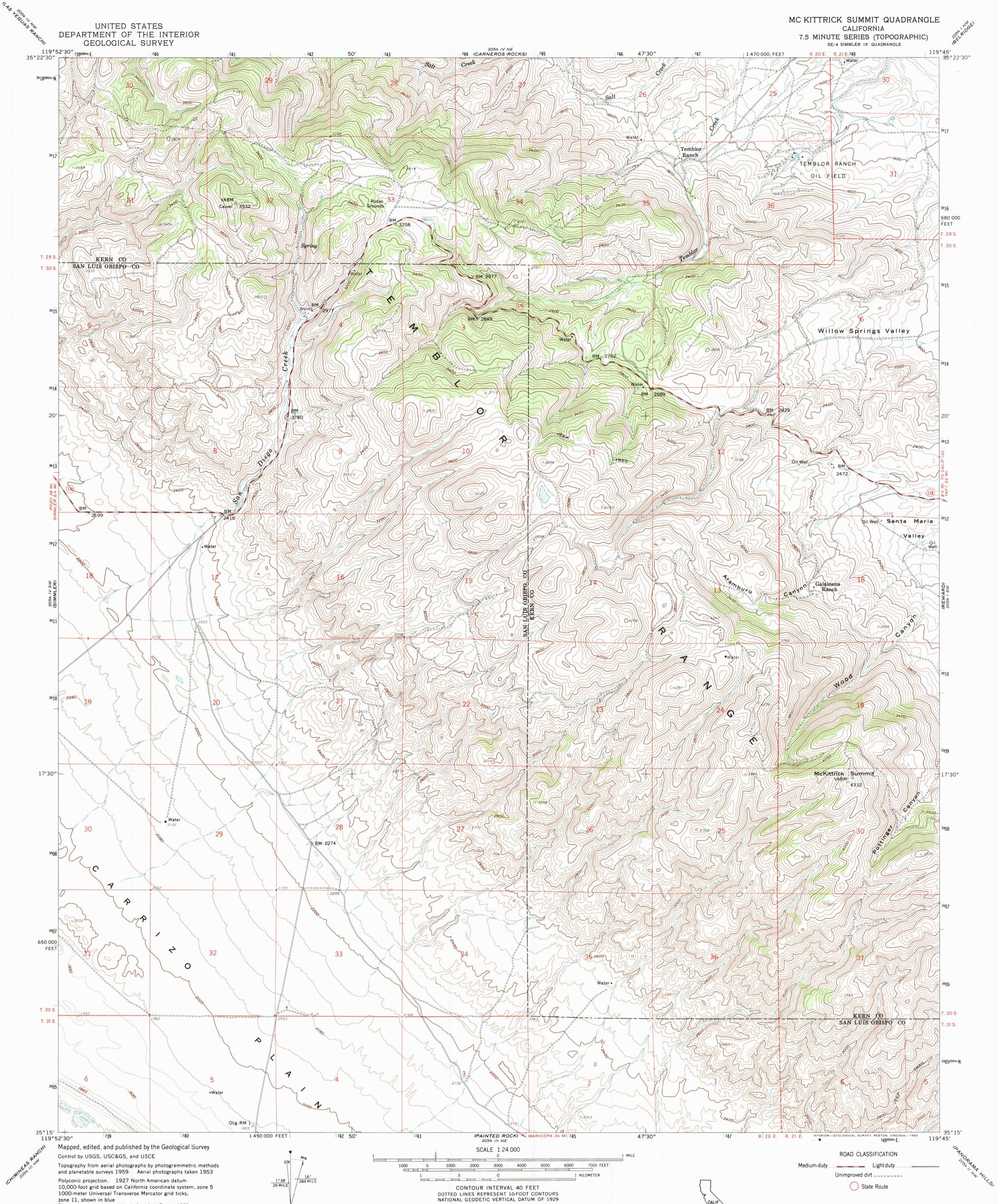
10,000-foot grid based on California coordinate system, zone 5 1000-meter Universal Transverse Mercator grid ticks, zone 11, shown in blue To place on the predicted North American Datum 1983 move the projection lines 6 meters north and 87 meters east as shown by dashed corner ticks Dashed land lines indicate approximate locations
