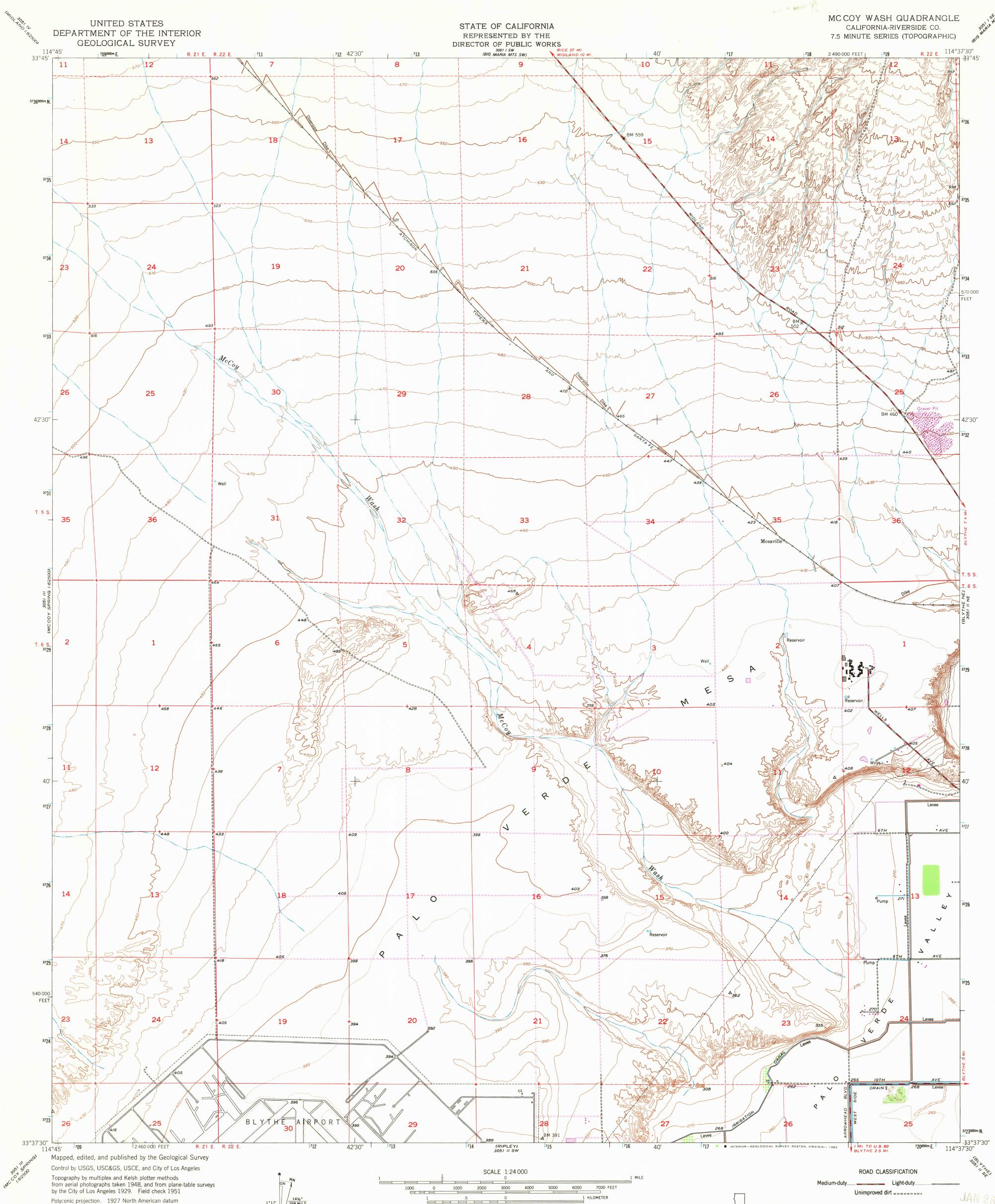
Polyconic projection. 1927 North American datum 10,000-foot grid based on California coordinate system, zone 6 1000-meter Universal Transverse Mercator grid ticks, zone 11, shown in blue To place on the predicted North American Datum 1983 move the projection lines 2 meters south and 73 meters east as shown by dashed corner ticks Revisions shown in purple compiled from aerial photographs taken 1970. This information not field checked
