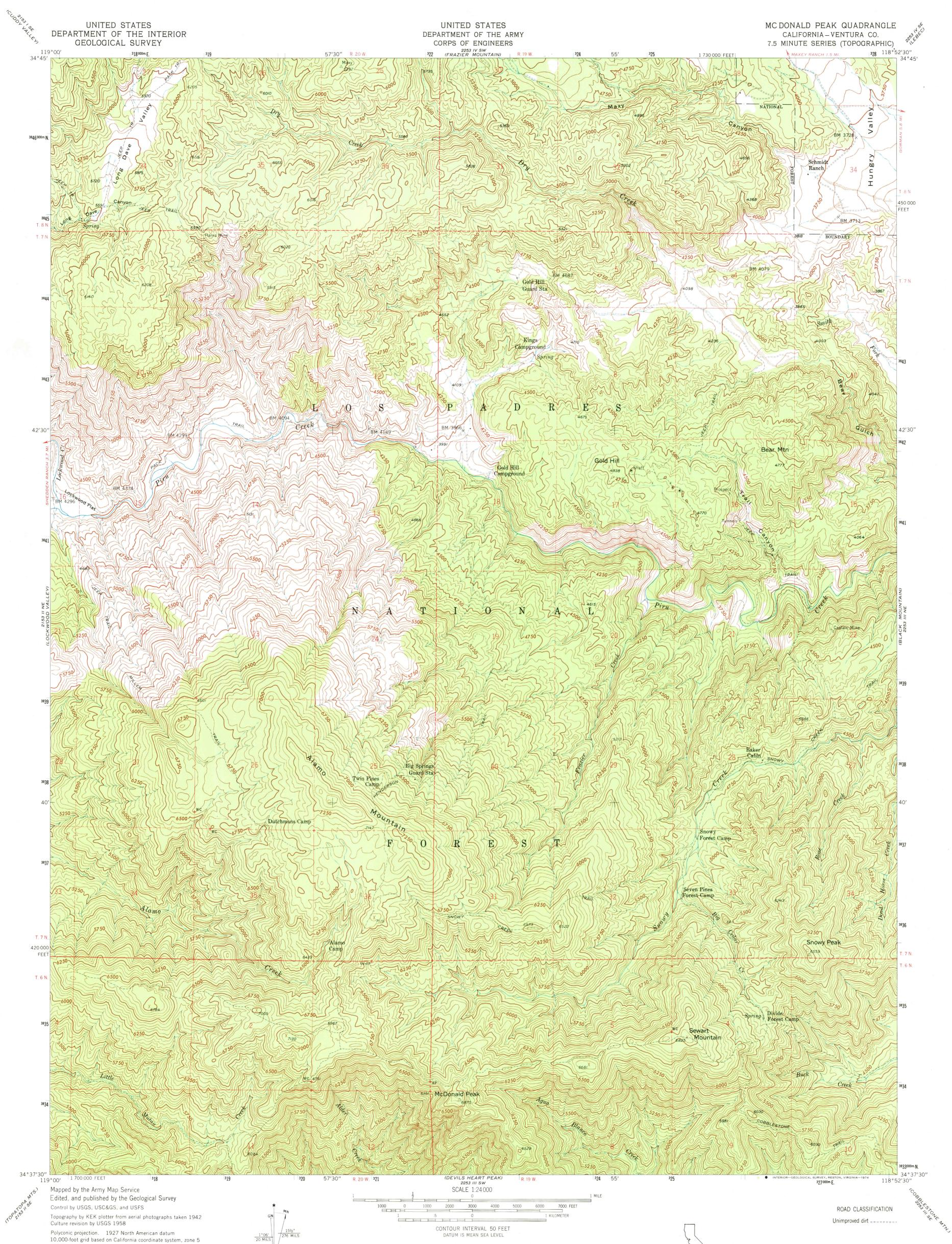
Polyconic projection. 1927 North American datum 10,000-foot grid based on California coordinate system, zone 5 1000-meter Universal Transverse Mercator grid ticks, zone 11, shown in blue
