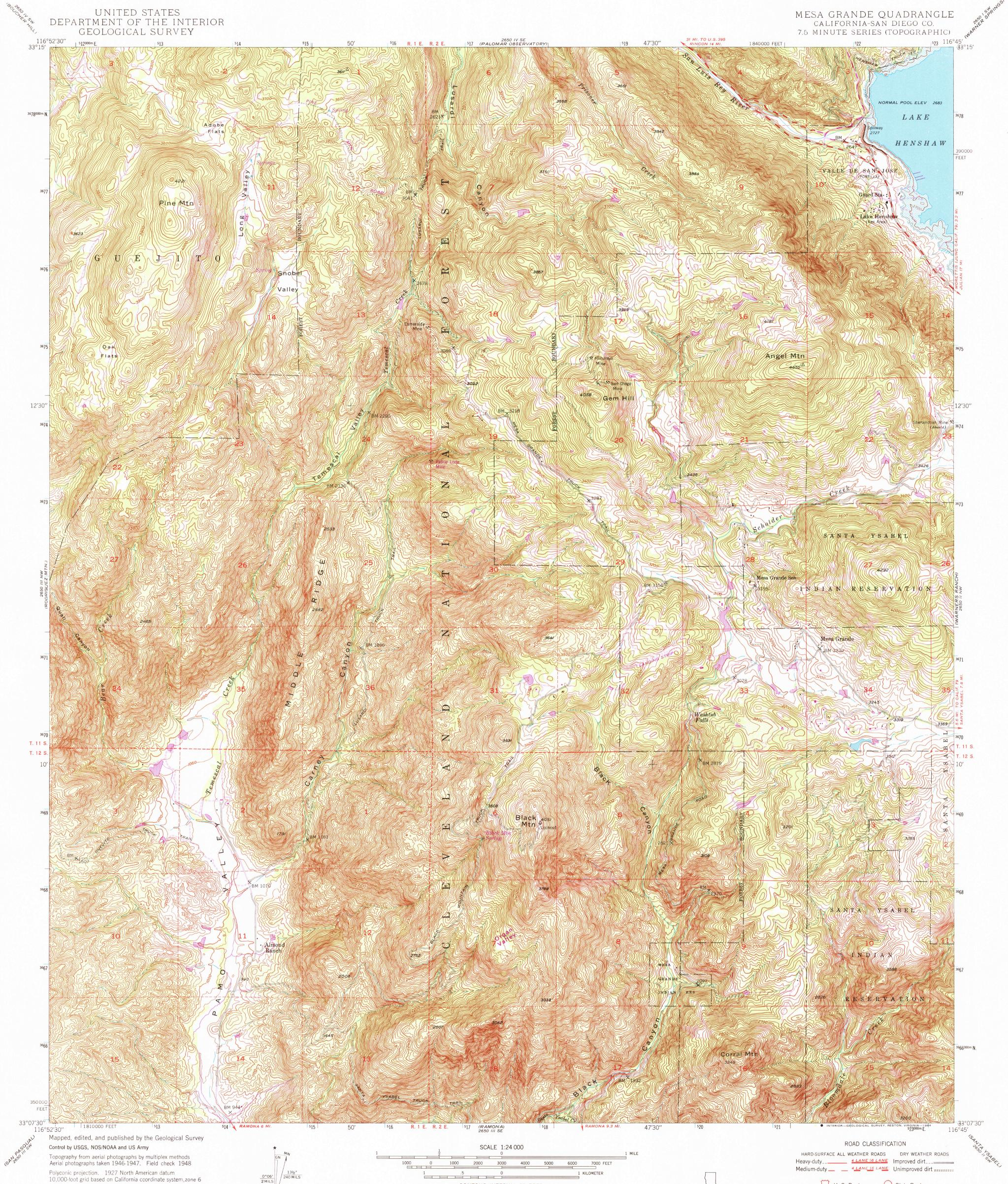
1000-meter Universal Transverse Mercator grid ticks, zone 11, shown in blue To place on the predicted North American Datum 1983, move the projection lines 2 meters south and 80 meters east as shown by dashed corner ticks Areas covered by dashed light-blue pattern are subject to controlled inundation There may be private inholdings within the boundaries of the National or State reservations shown on this map
