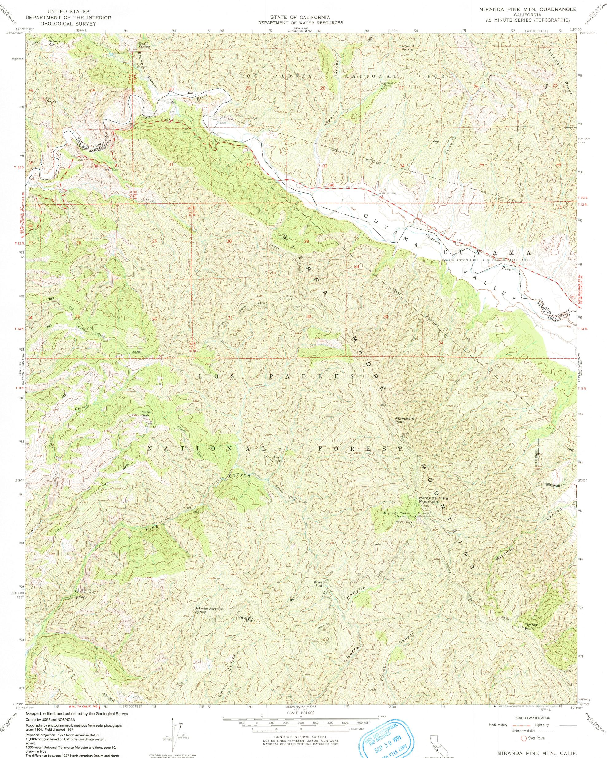
10,000-foot grid based on California coordinate system, zone 5 1000-meter Universal Transverse Mercator grid ticks, zone 10, shown in blue The difference between 1927 North American Datum and North American Datum of 1983 (NAD 83) for 7.5 minute intersections is given in USGS Bulletin 1875. The NAD 83 is shown by dashed corner ticks
