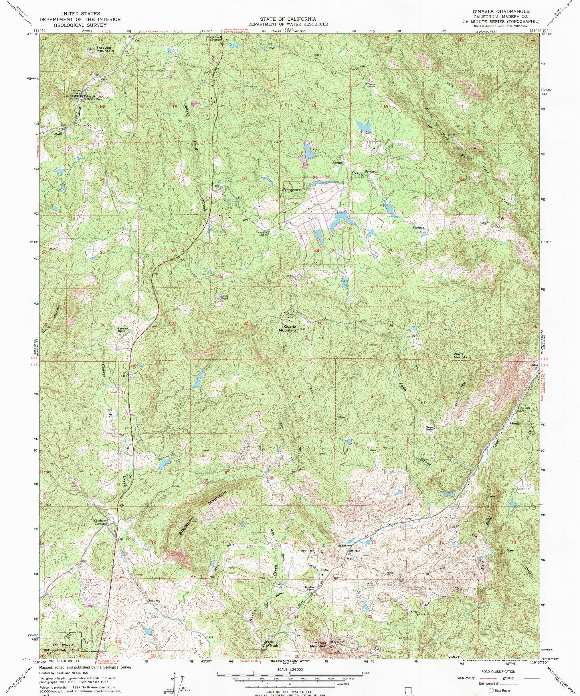
Polyconic projection. 1927 North American datum 10,000-foot grid based on California coordinate system, zone 3 1000-meter Universal Transverse Mercator grid ticks, zone 11, shown in blue
